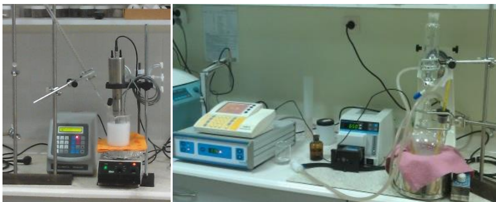
Figure 21. Experimental setup and instruments as US rod immersion (left) and US flow cell (right) for ultrasonic wave assisted precipitation and crystallization.
