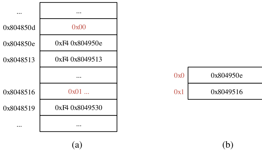
Figure 3.6: Rewriting Example: (a) Redirection Entries For Possible Jump Targets 0x804850d, 0x804850e, 0x80485013, 0x8048516, 0x8048519, (b) Redirection Entries In Extra Array
