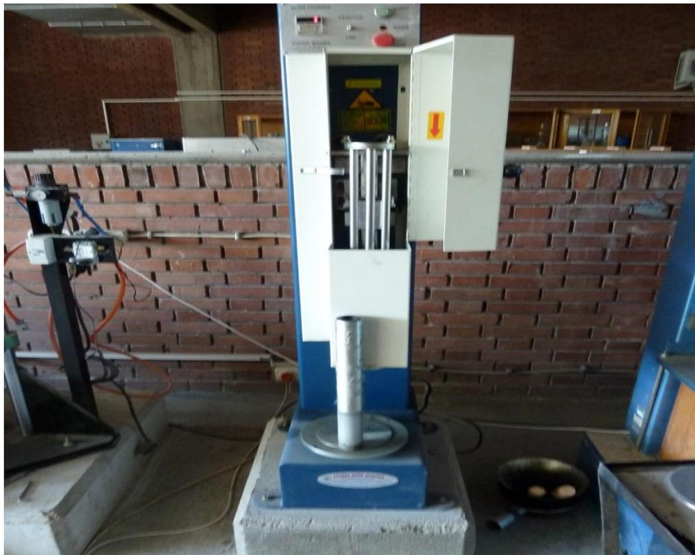
*Figure 3.14 Proctor Machine Used For the Research*
