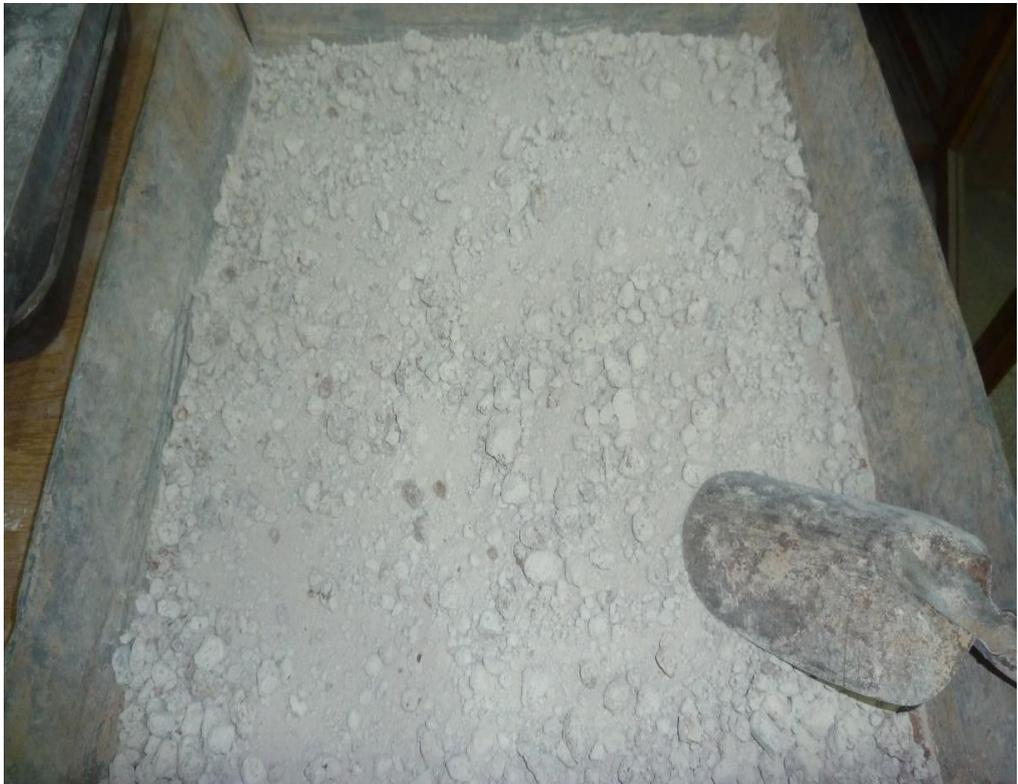
*Figure 3.16 Soft Soil and Borax Sludge Mixture*
