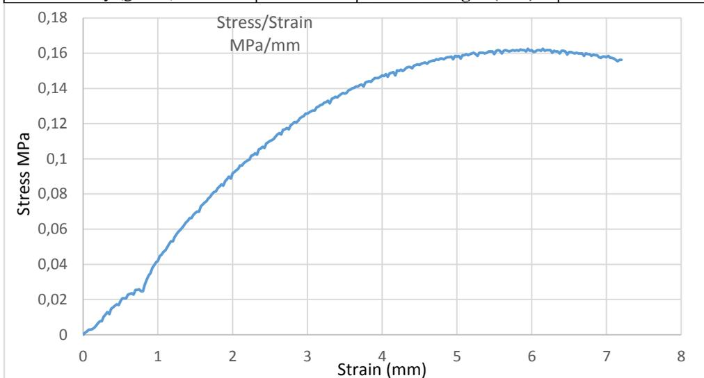
*Figure H.1 Unconfined Compressive Strength Test Data Sheets*
