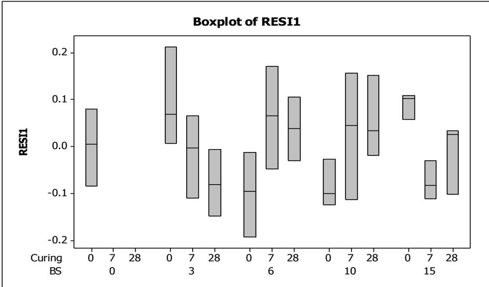
Figure 4.6 Boxplot of Residuals for California Bearing Ratio Test Results
