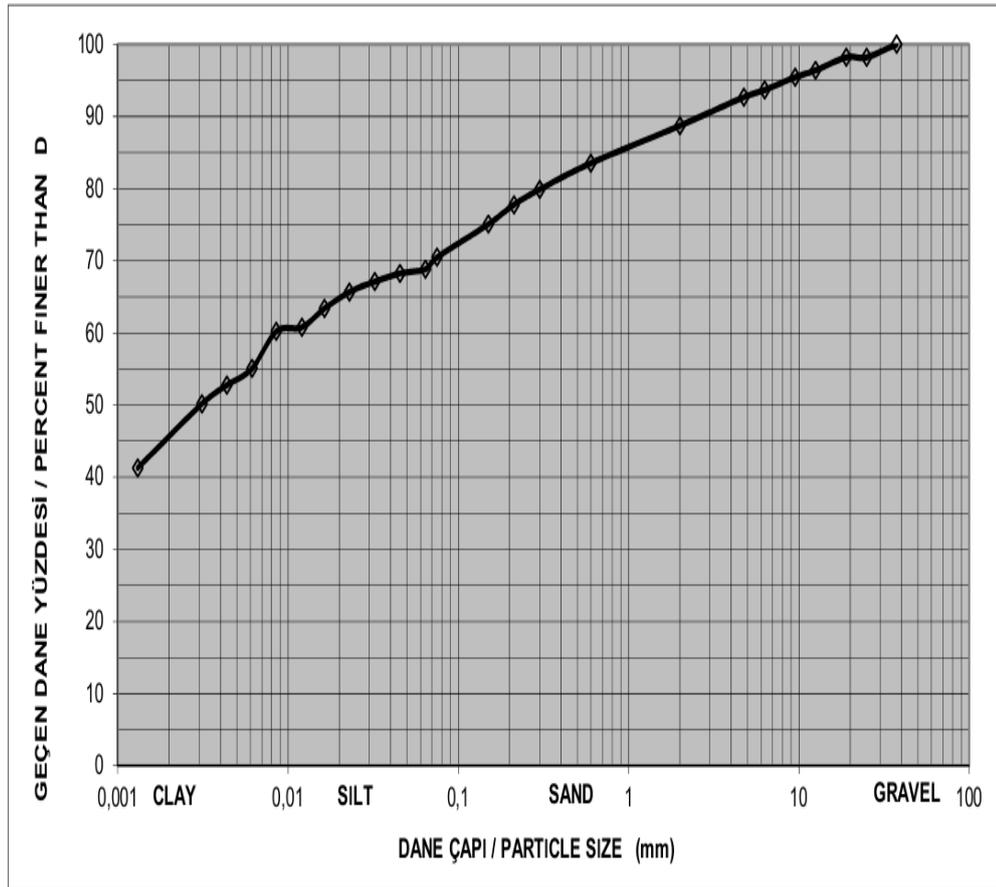
Figure 3.8 Soft Soil Gradation Curve
