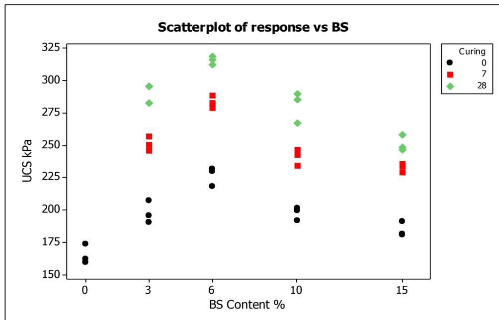
*Figure 4.10 Scatterplot of Unconfined Compressive Test Results*
