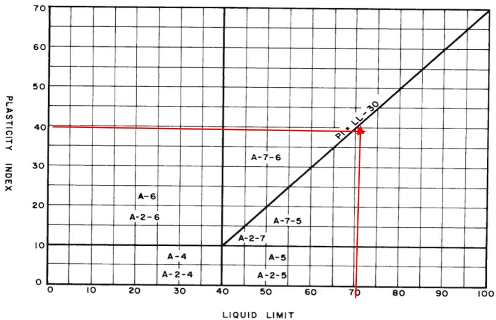
Figure 3.13 Plasticity Index for AASHTO Soil Classification (ASTM D3282, 2009)
