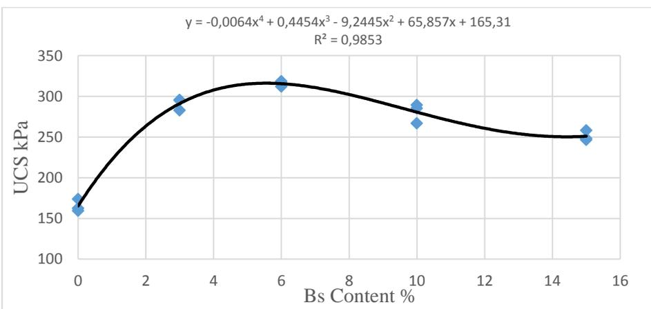
Figure 4.14 Polynomial Model for Unconfined Compressive Strength Test Results
