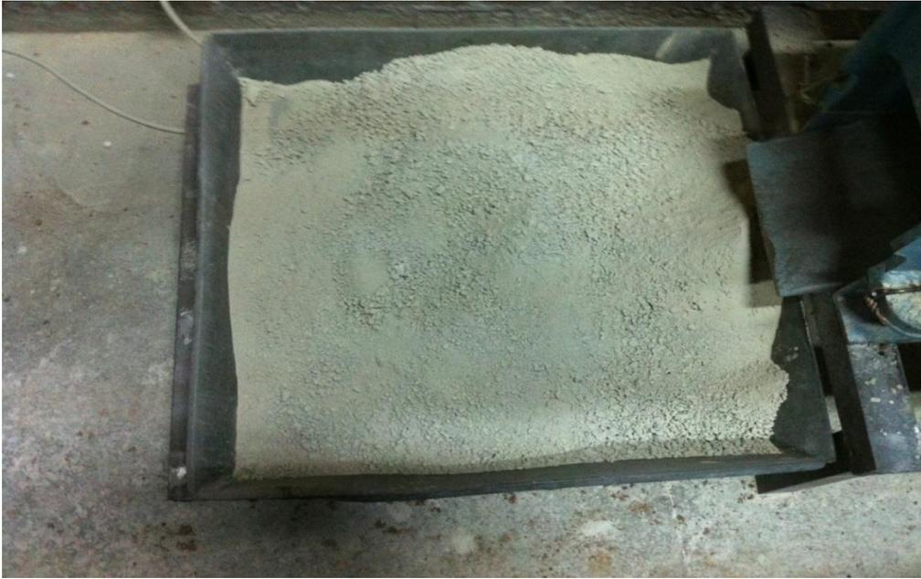
*Figure 3.4 Borax Sludge After Crusher*
