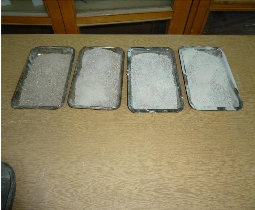
*Figure 3.21 Sieved Soil Samples for Unconfined Compressive Strength Test*
