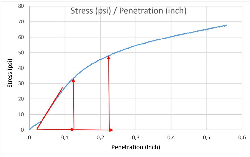
Figure 3.18 Stress/Penetration Curve
