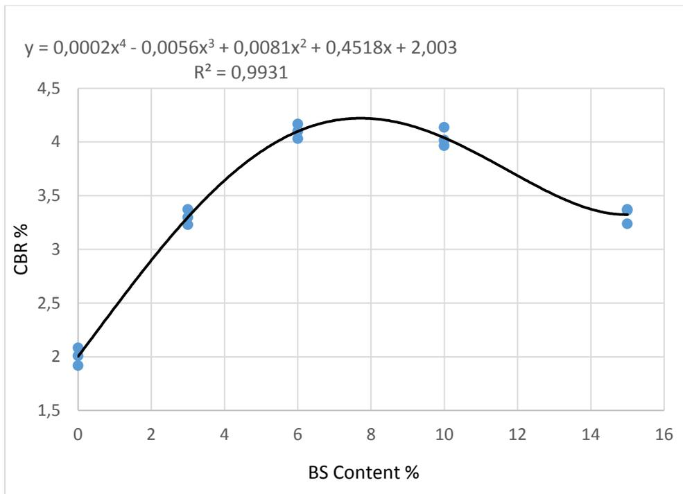
Figure 4.9 California Bearing Ratio Polynomial Model for 28 Days Curing
