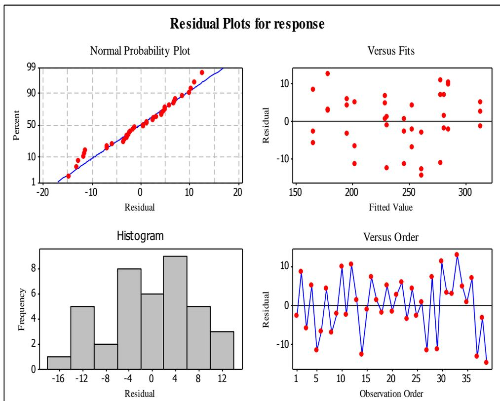
Figure 4.12 Residual Plots for Unconfined Compressive Strength Test Results
