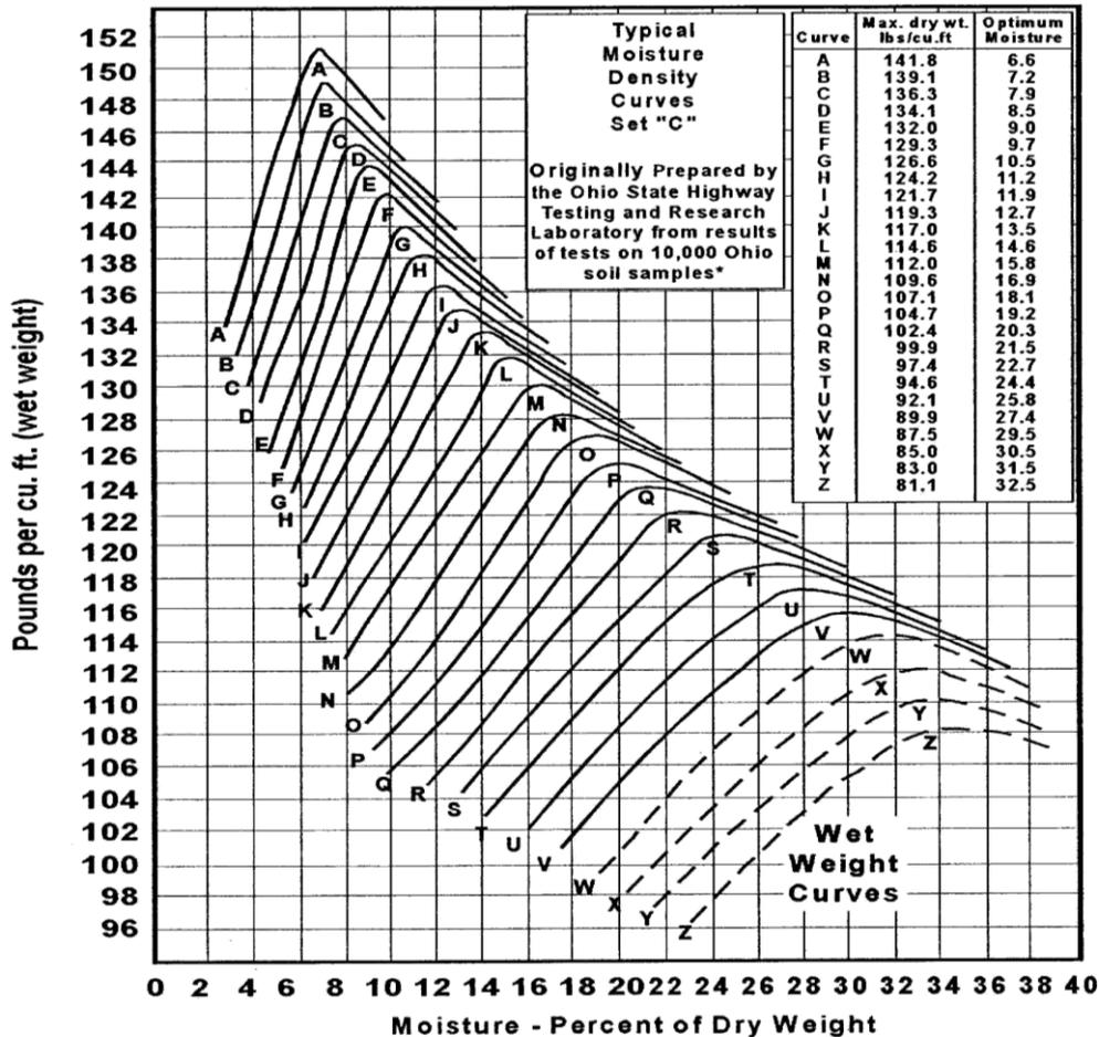
Figure 4.4 Family of expected wet density compaction curves, based on 18,000 compaction tests compiled by the Ohio DOT
