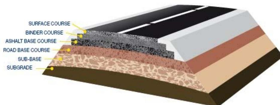
*Figure 1.1 Asphalt Pavement Structure and Subgrade*
