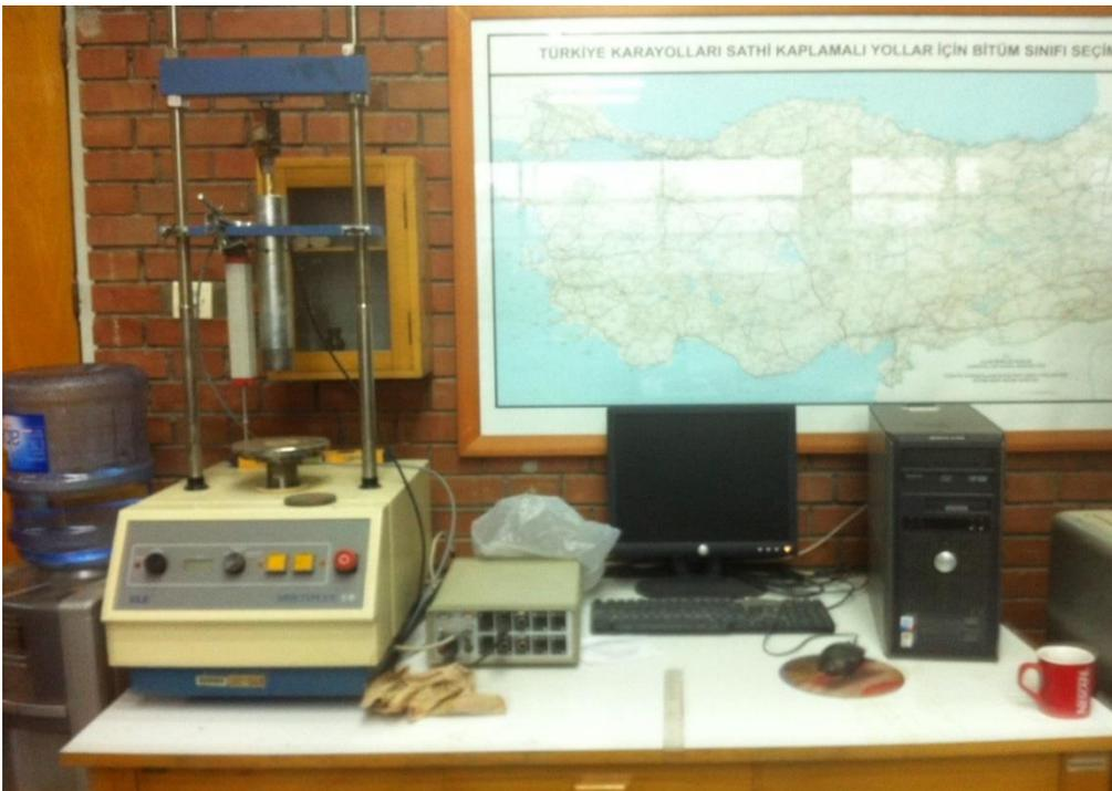
*Figure 3.17 California Bearing Ratio Test Device and Data Processing Equipment*
