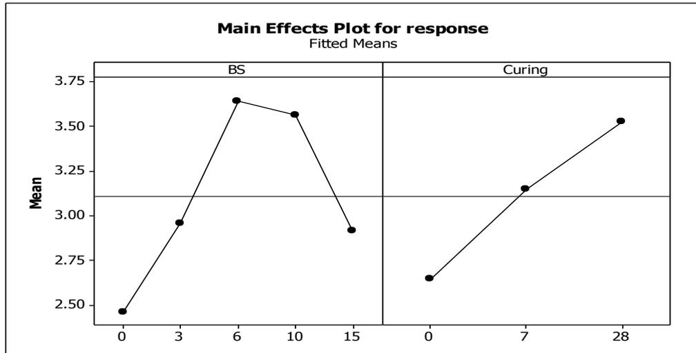
Figure 4.8 Factorial Fitted Means Graph of California Bearing Ratio Test Results
