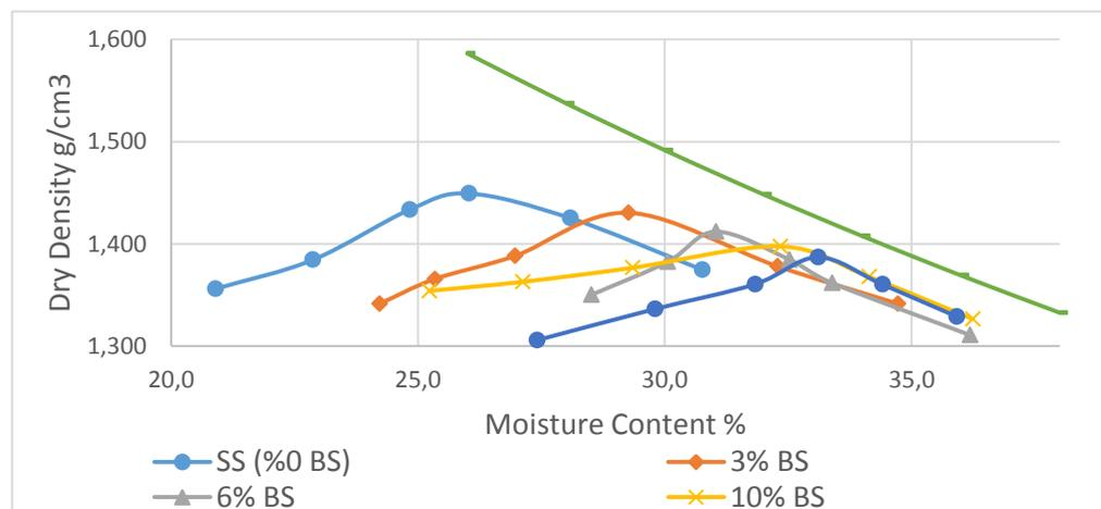
Figure 4.3 Proctor Moisture Curves
