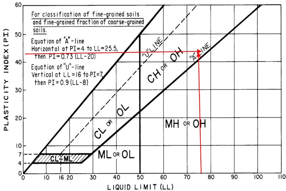
Figure 3.12 Plasticity Chart (ASTM D 2487-11)
