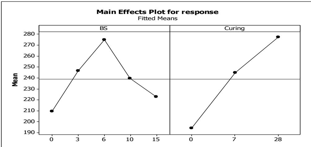
Figure 4.13 Main Effects Plot for Unconfined Compressive Strength Test
