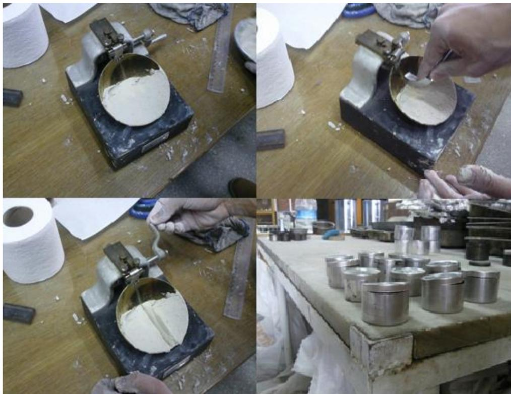
*Figure 3.10 Execution of Liquid Limit Test*
