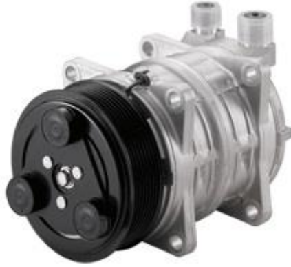
Figure 32 Piston Type with Swash Plate Compressor - VALEO TM16 [34]
