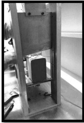
Figure 27 Slicing the propellant with guillotine
