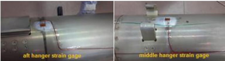
Figure 11. Locations of rosette strain gages on the DMS
