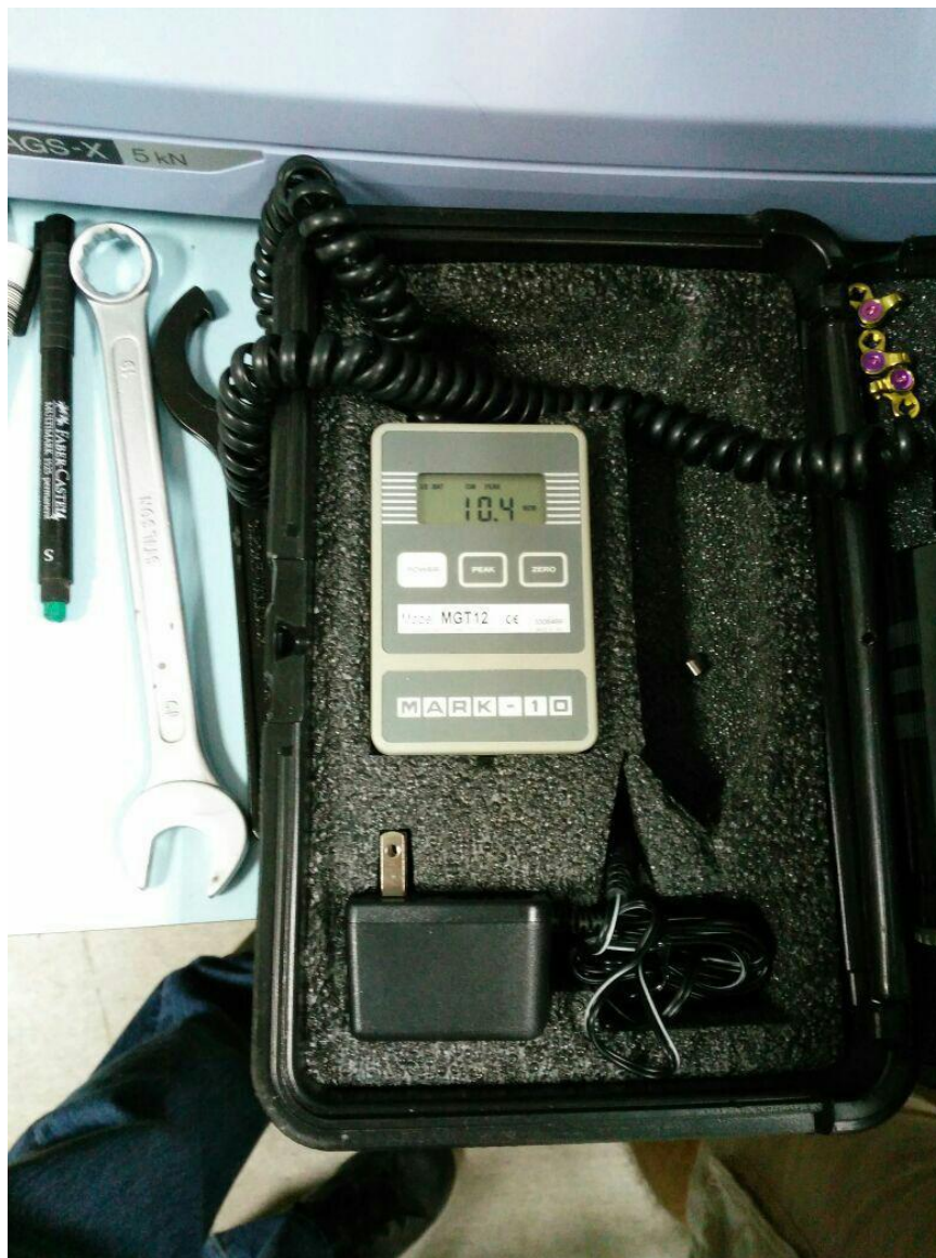
Figure 64: Image of Torque Meter after 10.4 N·cm Torque is Applied
