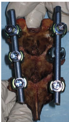
Figure 12: Left Side Control Rod and Right Side Reduced Rod (Kang, et al., 2014)
