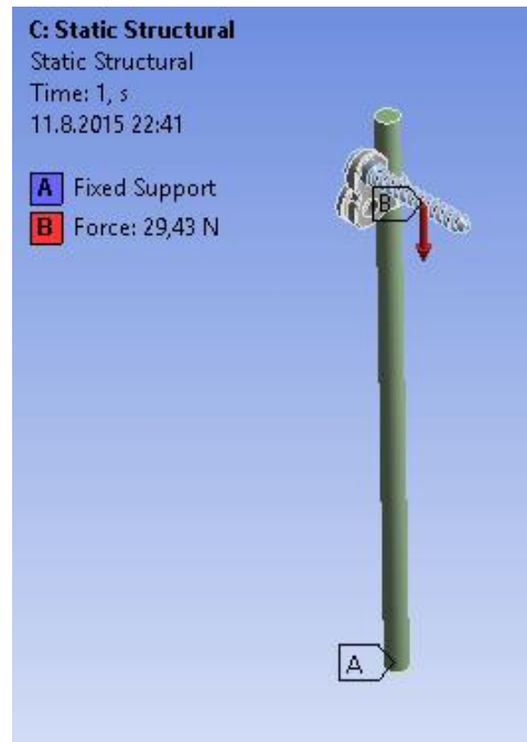
Figure 43: Boundary Conditions for Load Sharing Analysis
