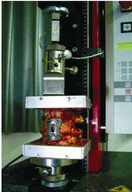
Figure 13: Anterior Lumbar Interbody Fusion+Anterior Lumbar Locked Screw Plate Specimen in Axial Compression Test (Liu, et al., 2014)
