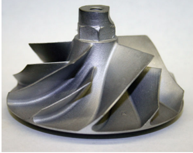
Figure 3.6: An Impeller with Splitter Blades [33]
