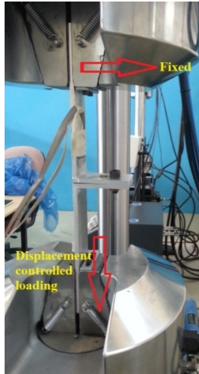
Figure 4.7 – Assembly of test machine and the test specimen
