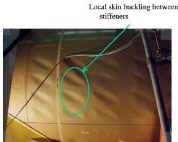
Figure 1.2 An example of buckling phenomena in aircraft fuselage [2]
