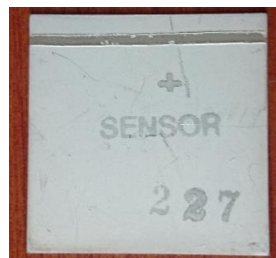
Figure 2.1 Sensor Technology BMP500 (PZT - Lead Zirconate Titanate)
