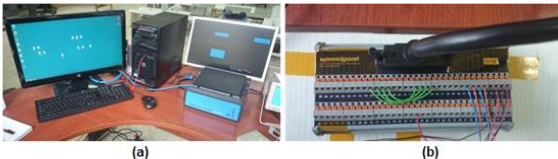
Figure 2.14 Data Acquisition System (a) Host PC and xPC Target Machine (b) Terminal Board
