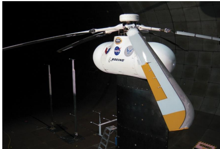
Figure 1.2 The Smart Rotor, Blade, and Flap in the Tunnel [14]
