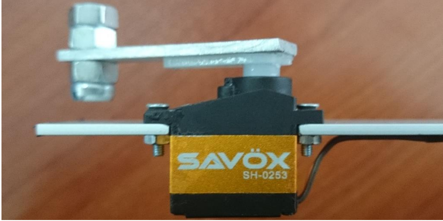
Figure 2.8 Top View of the Mass Variation Mechanism
