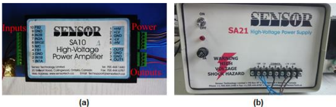
Figure 2.16 Amplification System (a) SA10 Power Amplifier (b) SA21 Power Supply
