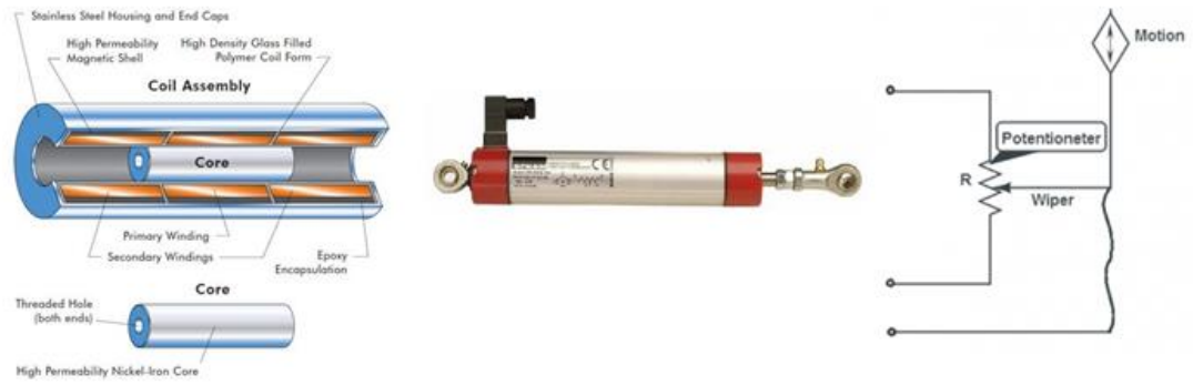
Figure 36 Inside and Outside View of LVDT
