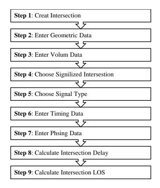
Figure 2.2 The step of LOS calculation according to Synchro v.9
