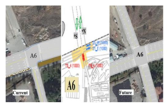
Figure 6.3 Current and future geometry of "A6" intersection
