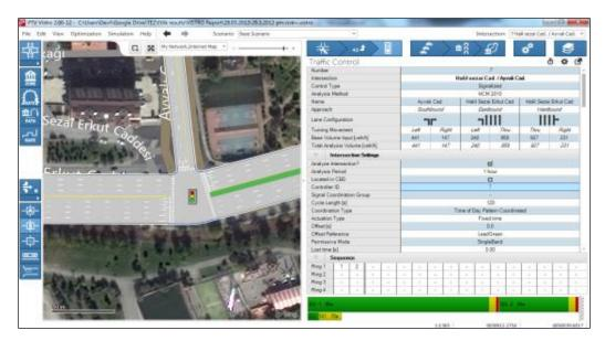
Figure 5.11 Screenshot of signal and phase time input for "A2" intersection in Vistro
