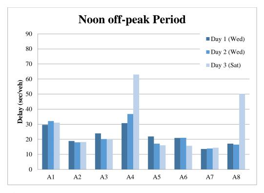
Figure 5.15 Total average delays in Noon off-peak period of all intersections in three days by Vistro
