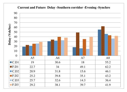
In general, the results showed that the Delay and LOS of all intersections increase in all days. Also, the results by Vistro generally showed higher delay than Synchro, because of their embedded delay function. That is why, the Vistro results seem more reasonable than Synchro.
