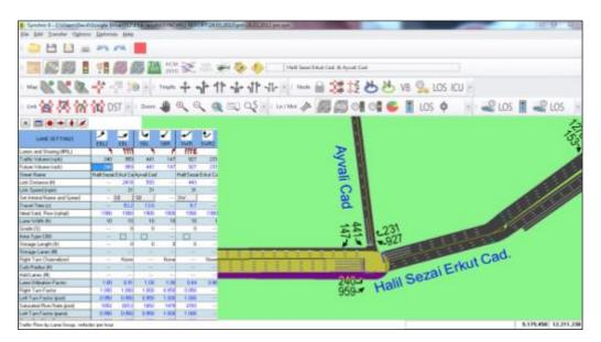
Figure 5.3 Screenshot of gemoetry and volume input for "A2" intersection in Synchro
