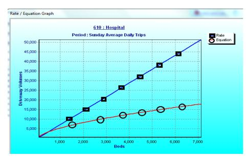
Figure 5.20 Difference between equation and rates in ITE 2008
