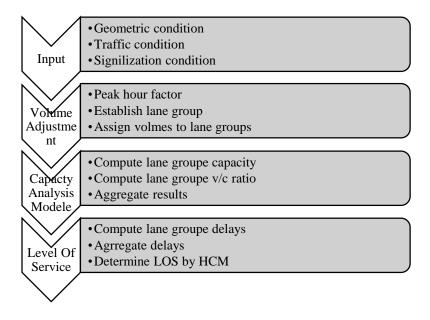
The HCM version 2010 proposed the method to determining control delay, which is based on the direct observation of the vehicle in queue counts at signalized intersection. The delay that was accomplished by all the vehicles that arrive during the examination period is demonstrated as an average control delay, which is presented in Equation 2.1.
