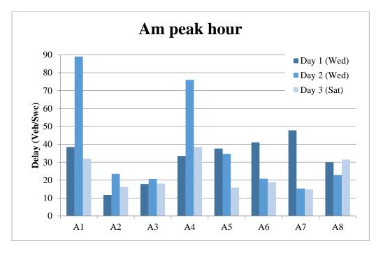
Figure 5.14 Delays in AM peak hour of all intersections in three days by Vistro
