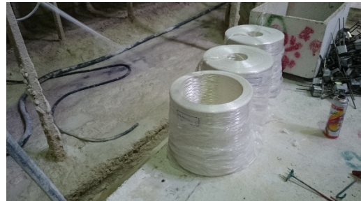
(b) Glass fiber filaments used in GRC
