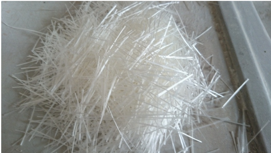
Figure 1: Appearance of chopped alkali resistant glass fibers
