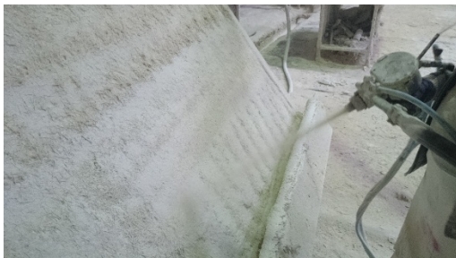
(c) Air gun used for spraying the premix
