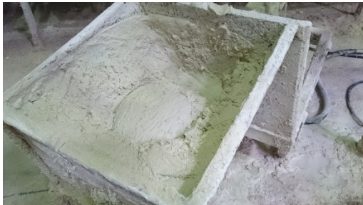
(a) The slurry being mixed in the tank
