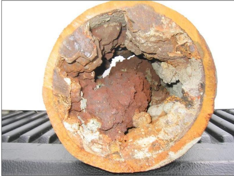
**Figure 2.9** Aging of Pipe (Web 5)
