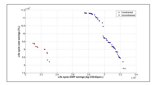
Figure 6.8. Non-dominated Solutions for Insulation Thickness Limitation Case
