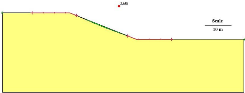
Figure 4.30 Failure surface from Slope/W analysis
