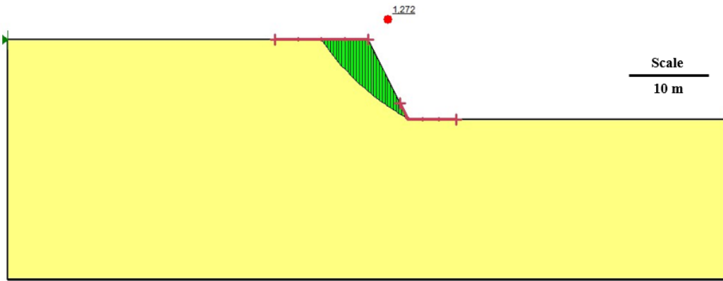
Figure 4.16 Failure surface from Slope/W analysis (c-phi Soils)
