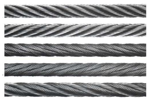
Figure 53. Strand lay configurations [24]
