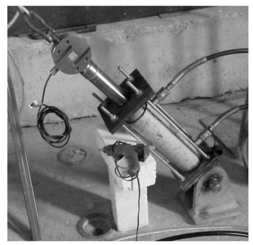
Figure 62. Cable - load cell - hydraulic jack assembly
