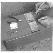
8. Soldering and fixing the cables
