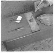
7. Soldering the strain gauge ribbons
