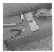
3. Positioning of the strain gauge with tape
