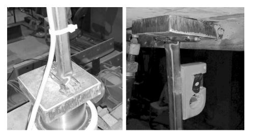
Figure 34. End crushing of the column before plastic buckling load is reached
