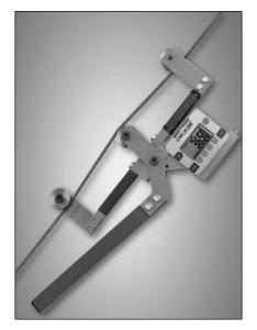
Figure 5. "Check-Line Cable Tension Meter" [6]
