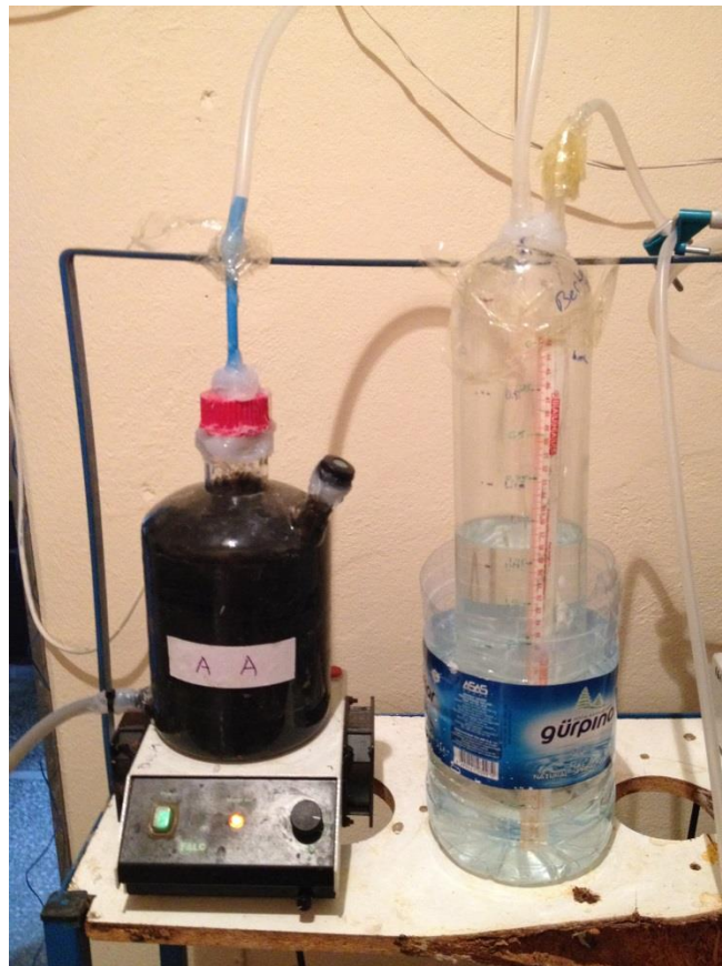
Figure 3.4: The reactor setup including the gas collection unit and the stirrer.
