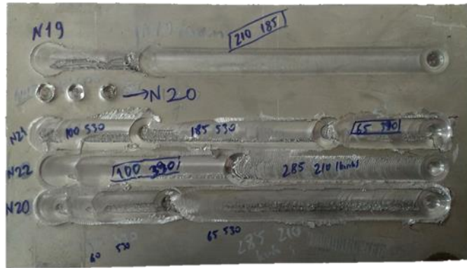
Figure 47. Surface appearance after the trials with the tool triflute.
