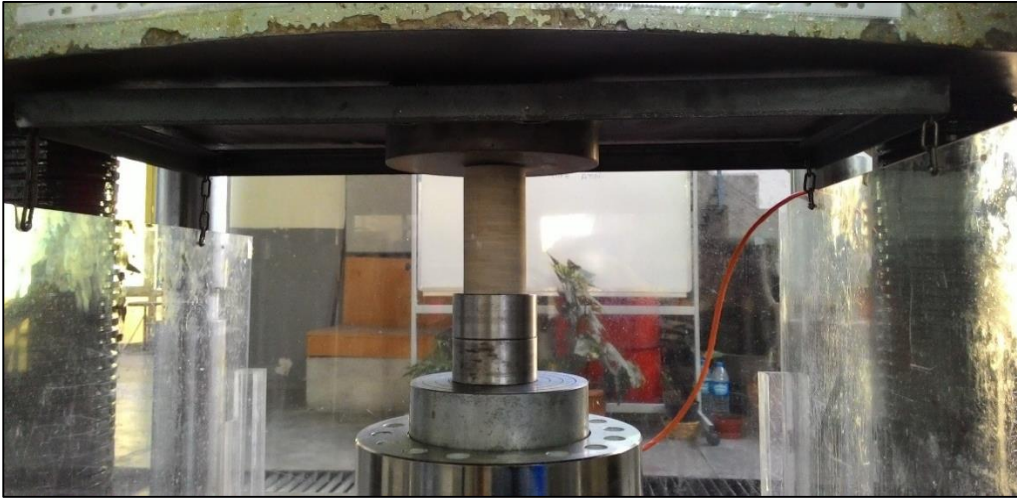
Figure 3.14 Illustration of UCS test
