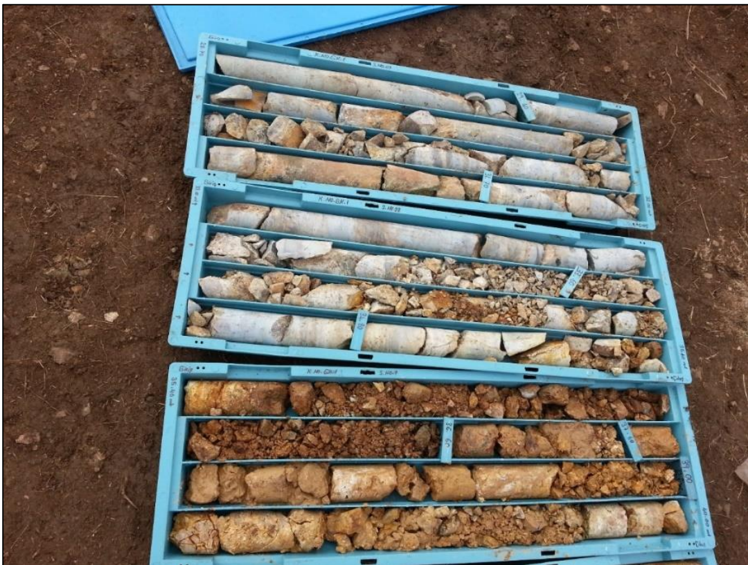
Figure 3.11 An example of drillhole core in Bizmişen region (Karpuz, et al. , 2014)
