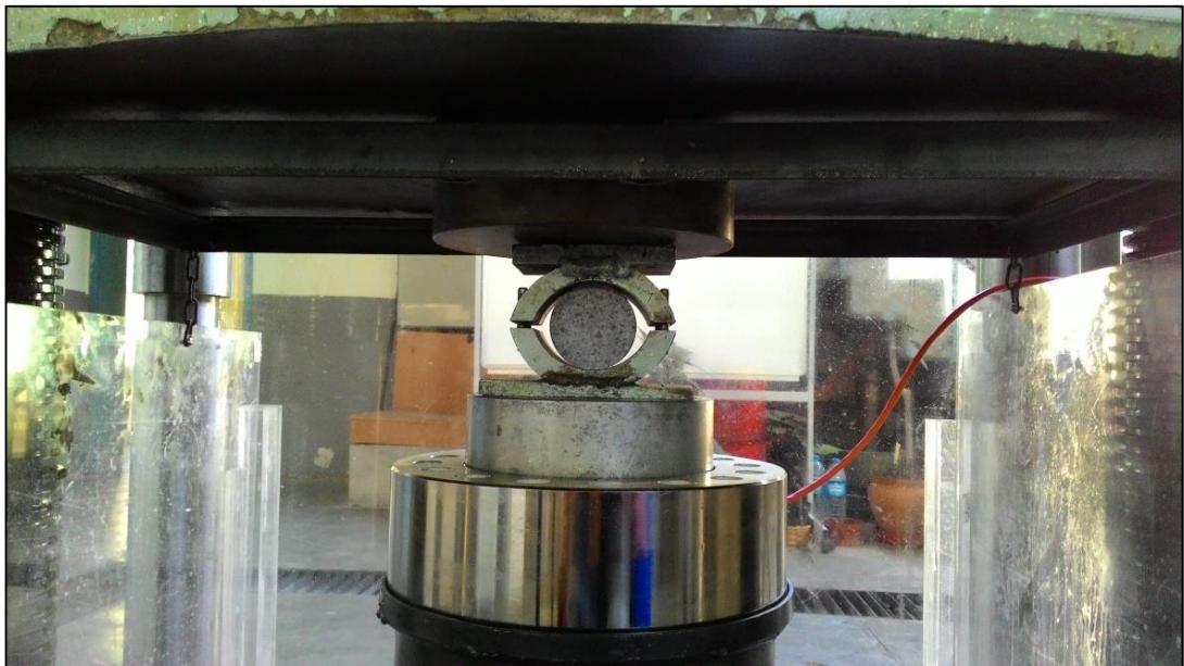
Figure 3.16 Illustration of indirect tensile strength test
