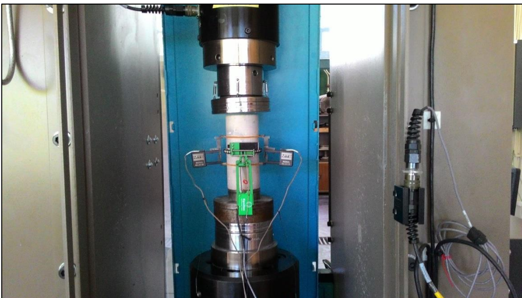
Figure 3.15 Illustration of Static Deformability Test
