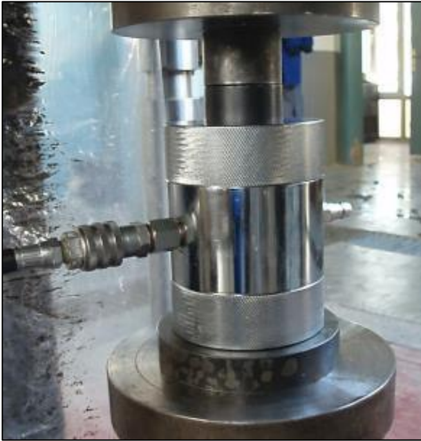
Figure 3.17 Illustration of triaxial compression test
