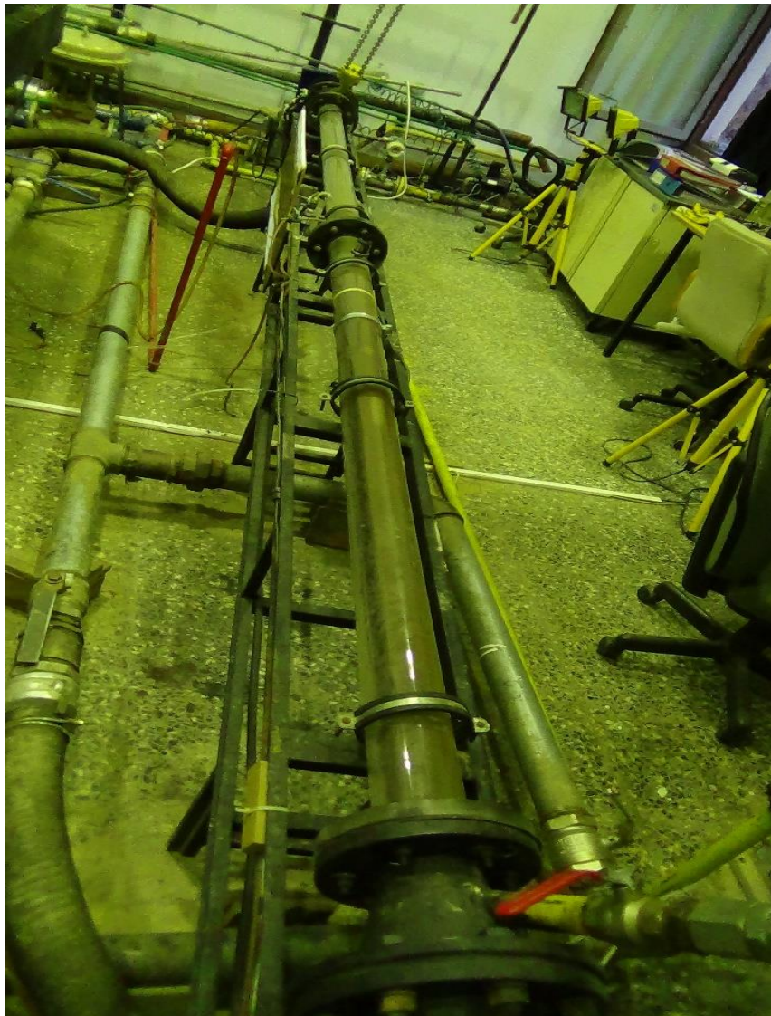
Figure 3. 2 METU-PETE Cuttings Transport Flow Loop
