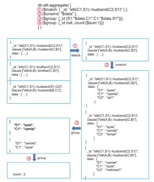
Figure 4.8: Aggregation pipeline for Calculating Support
