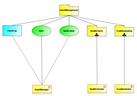
Figure 4.6: Decomposition of EventManagement package
