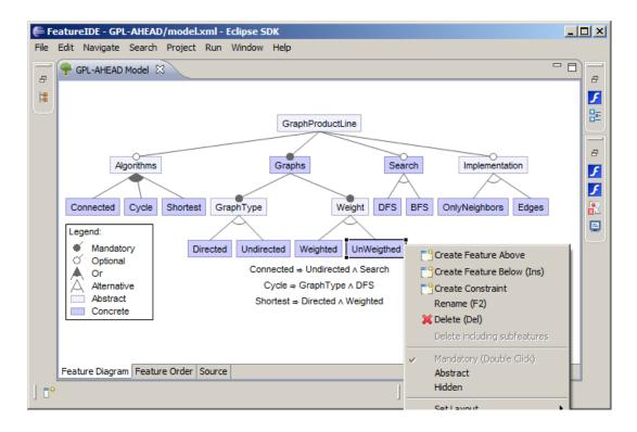
Figure 3.3: FeatureIDE screenshot that displays a feature model (from [41]) and constraints on the feature model.
