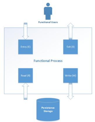
Figure 2.5: Data movements of COSMIC method (from [15])
