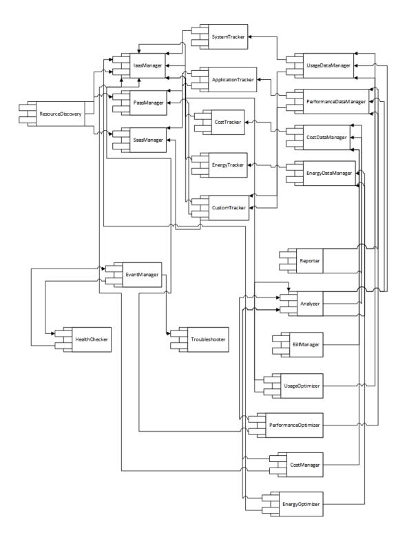
Figure 4.8: Component relationship diagram of cloud management system
