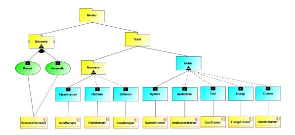
Figure 4.4: Decomposition of Monitor package
