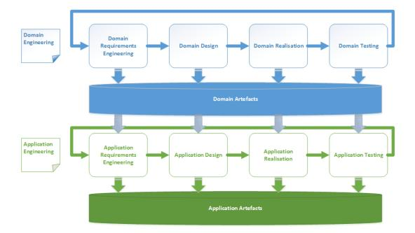
Figure 2.2: SPLE phases (adapted from [37])
