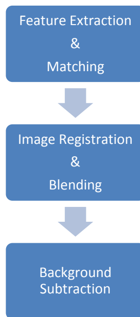
Figure 1: Steps for Pan-Tilt Camera Motion Detection System
