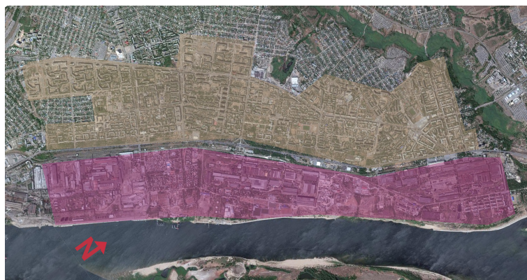
Figure 3.4: Stalingrad -Volgograd- Satellite Image. Stalingrad was a Soviet City which was designed by Miliutin according to Linear City principles; residential and industrial zones which are diverged by main highway and railway line settled parallel to each other by River Volga. Another remarkable point is areas on the west side of old residential area which were built up after collapse of Soviet Union. Urban land was divided to small parcels and buildings are smaller than the buildings of old residential area. Non-organized market mechanism slogs on to built large projects.
