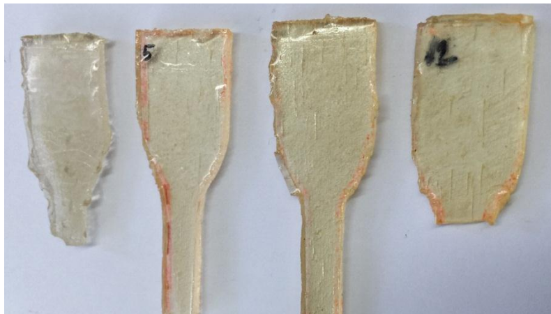
Figure 3.2: Physical Appearance of Neat Polyester Resin Irradiated by Low Dose Rate Gamma Source with Increasing Doses
