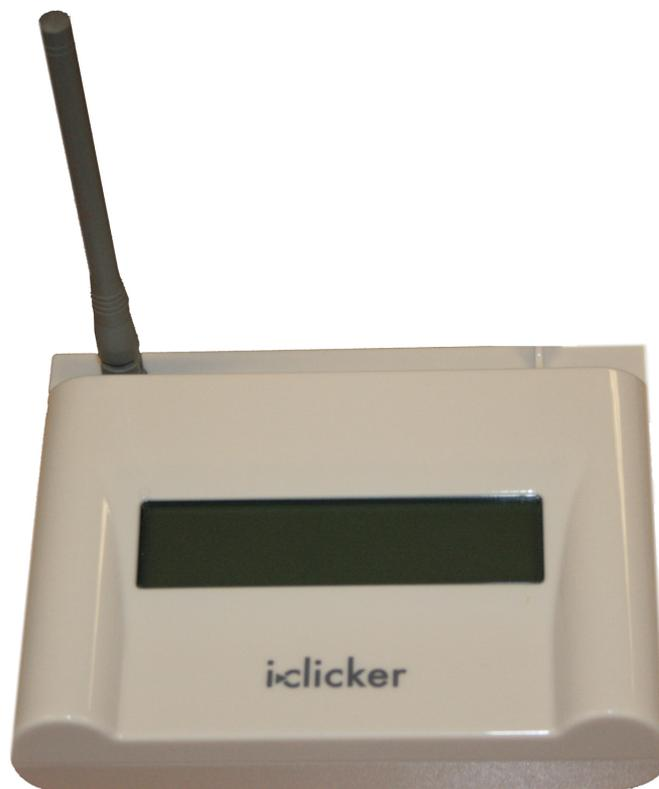
Figure 1.3 *A Receiver for SRS*
