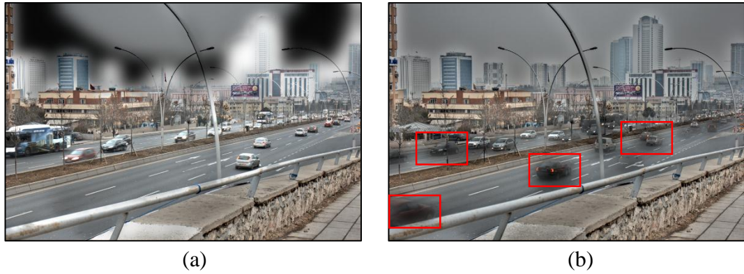
Figure 4-20 Final Enhanced Images of Input Set 4, when Reference Image Selection by Evaluating, (a) Well-Exposedness, (b) Percentage of Saturated and Unsaturated Pixel
