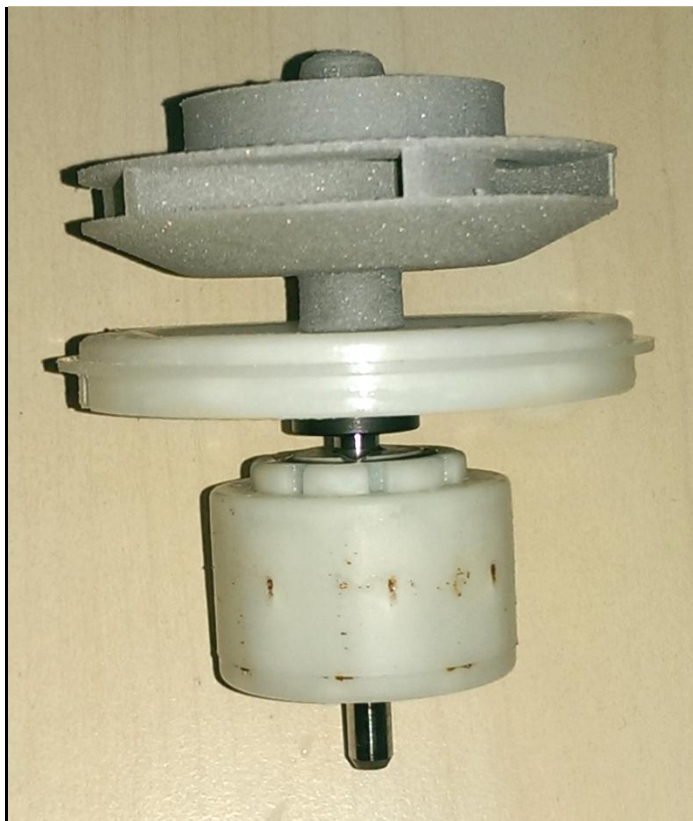
Figure A.4- Prototype of designed impeller assembled to shaft and wet rotor
