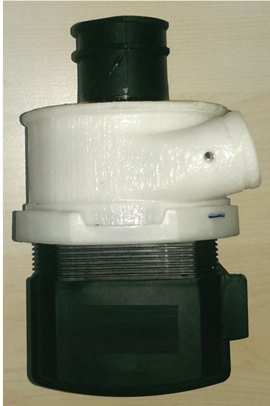
Figure A.9- Prototype of designed volute assembled to electric motor and inlet hose (with water-resistant glue on it)
