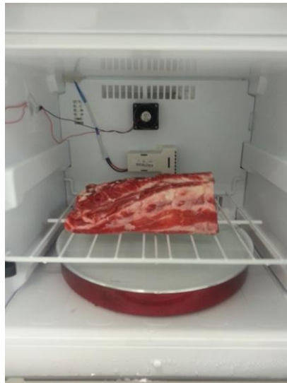
Figure B.2 Aging of meat in dry aging unit of refrigerator (Arçelik A.Ş, Eskişehir, Turkey)
