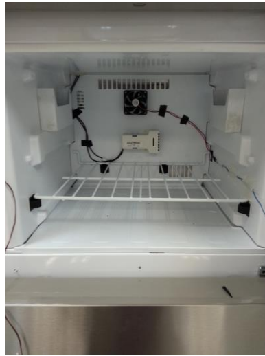
Figure B.1 Prototype of dry aging unit (Arçelik A.Ş, Eskişehir, Turkey)
