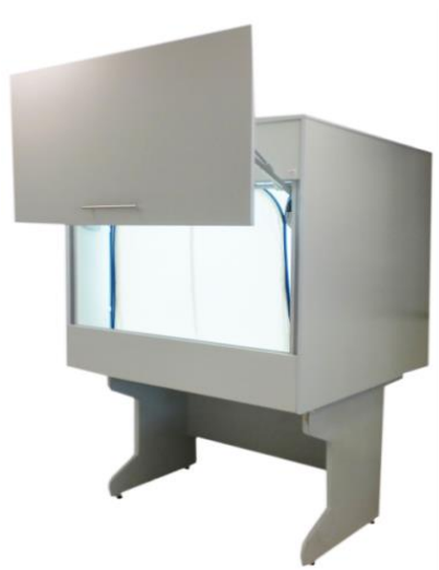
Figure B.4 The cabinet and lighting system for image processing
