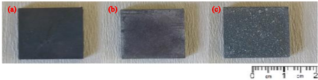
Figure 14: Plates coated 1mM Sr added solution: (a) Plate at 9 th day of immersion, (b) Plate at 14 th day of immersion; (c) Plate at 18 th day of immersion.
