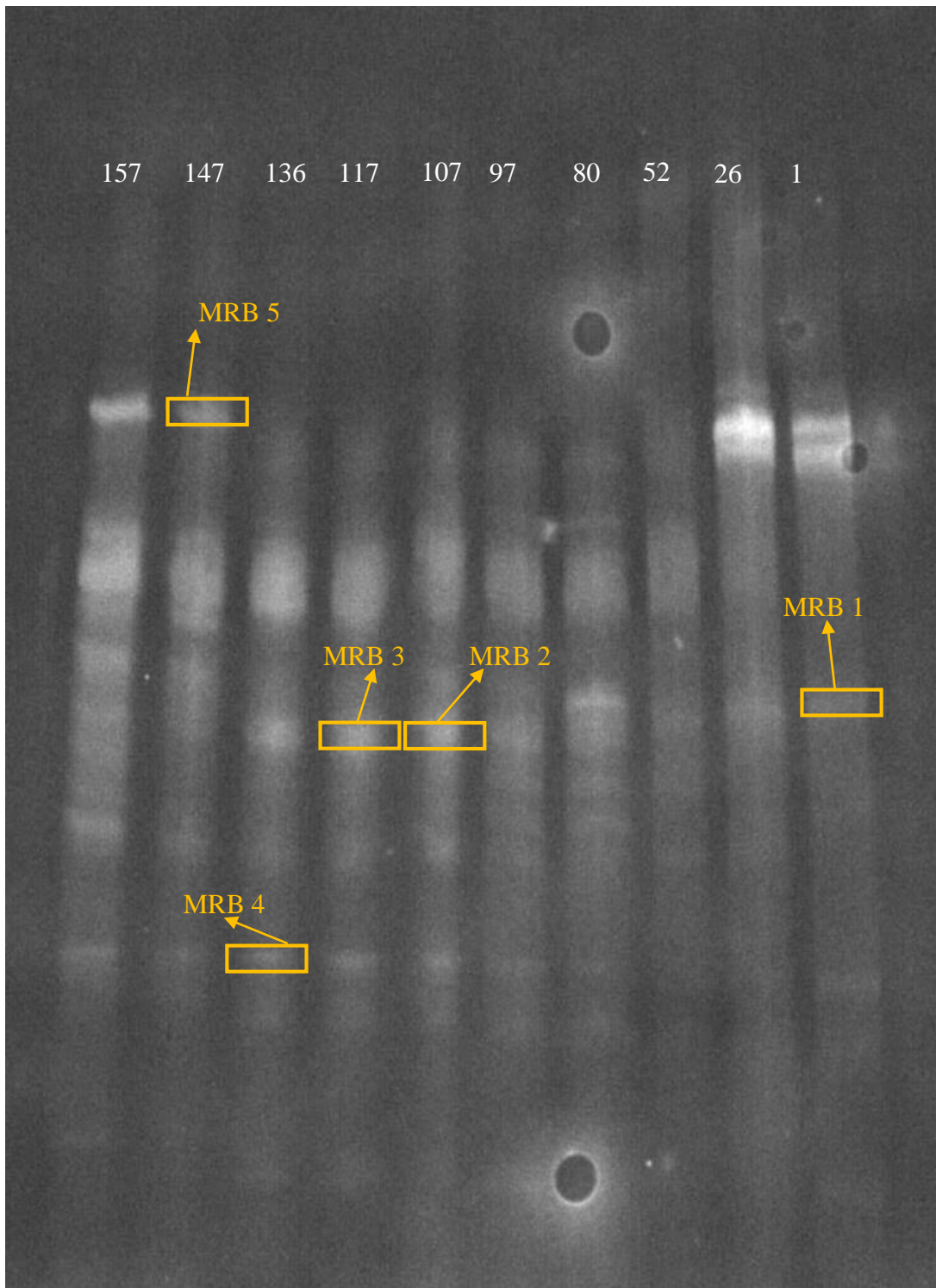
Figure 4-8 DGGE analysis image of all Bacteria (1-157 on each lane indicates the operational days when the sludge samples were taken and the bands marked with “ ” and “MRB” indicated the bacterial species (bands) used for sequence analyses)
