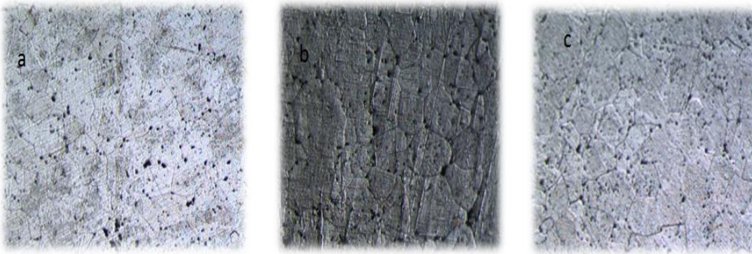
Figure 4-26: Micro hardness and microstructure of aging times at 240°C, a. after 90 min, b. 180 min and c. 360 min aging. X100
