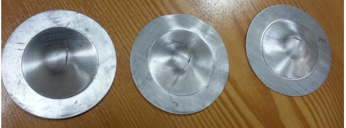
Figure 4-31: Erichsen test specimens
