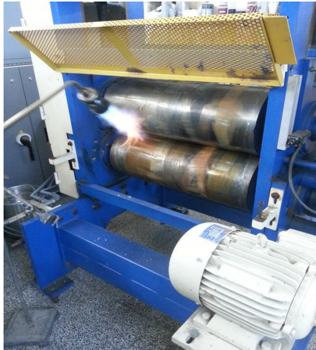
Figure 3-2: Rollers heated to about 70°C to prevent edge cracking
