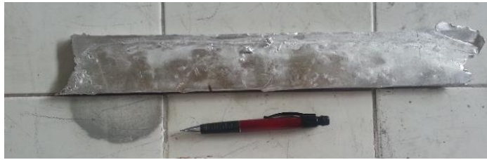
Figure 4-1: Experimental as-cast 6.7 mm AA6111 plate
