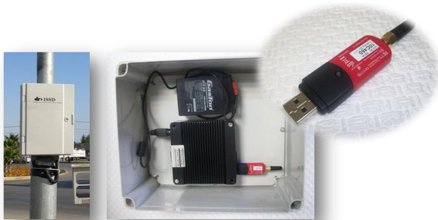
Figure 11 Class 1 type Bluetooth reader device with antenna (range 300m) used in the Etlik and ESE corridors case studies
