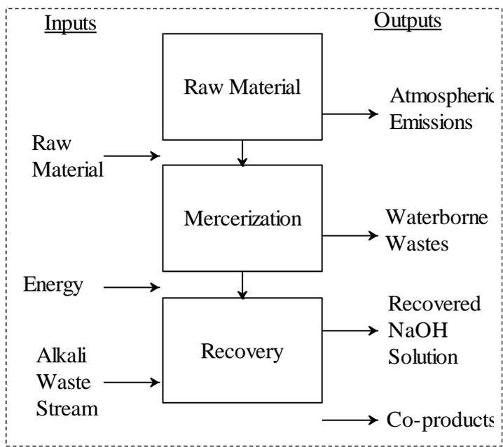
Figure 11. System under consideration for evaporative recovery
