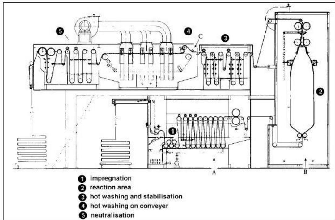
Figure 4. Example of mercerizing equipment for knitted fabric [2]
