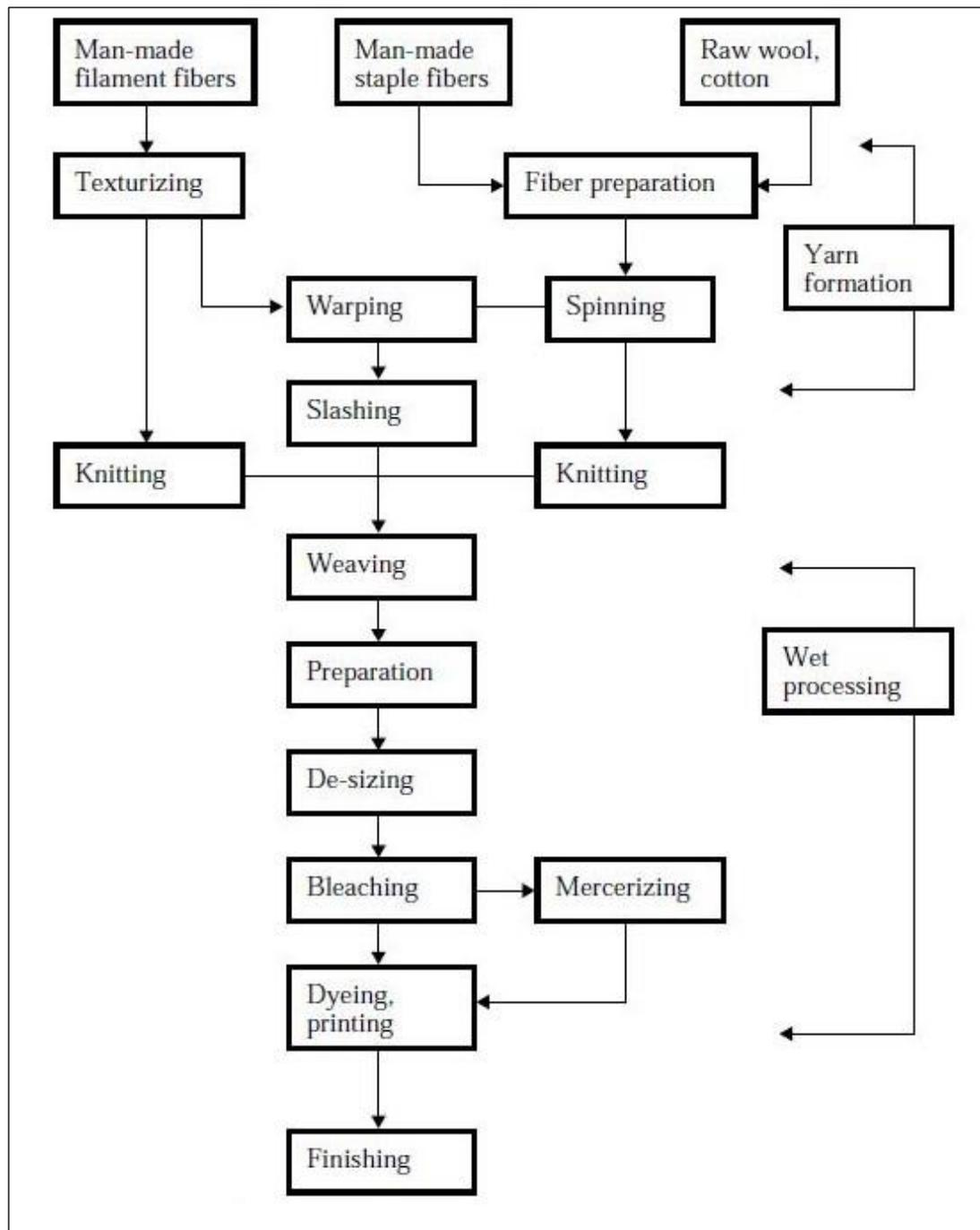
Figure 1. Processes for cotton processing textile mill [3]
