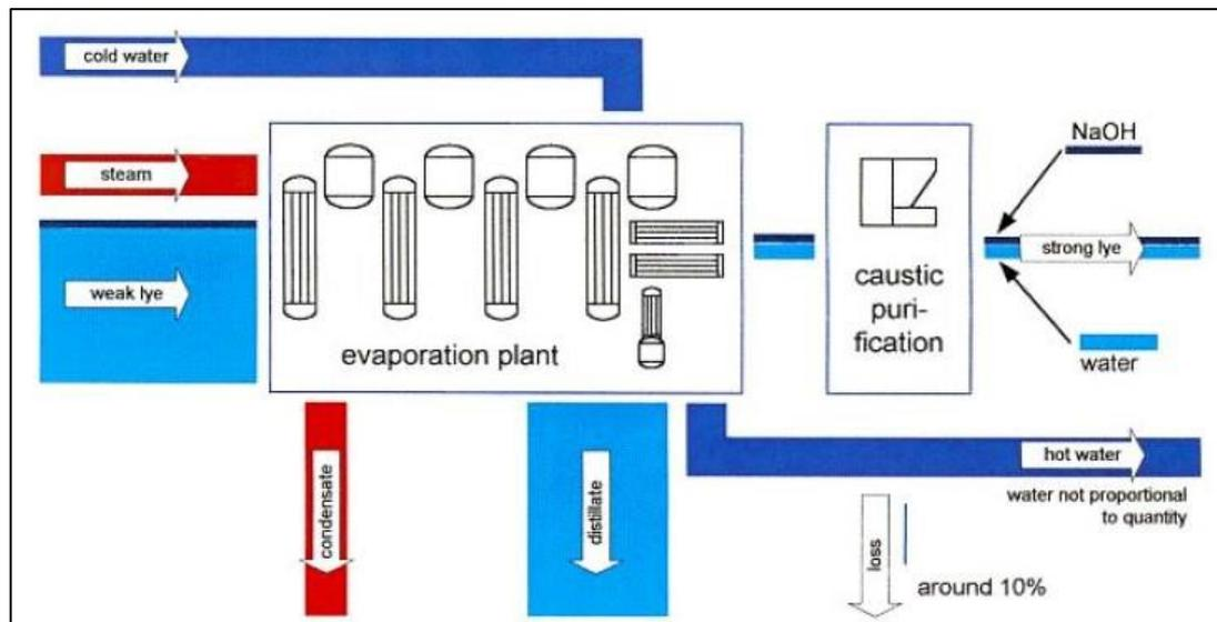
Figure 5. Scheme of evaporation plant for caustic recovery [2]
