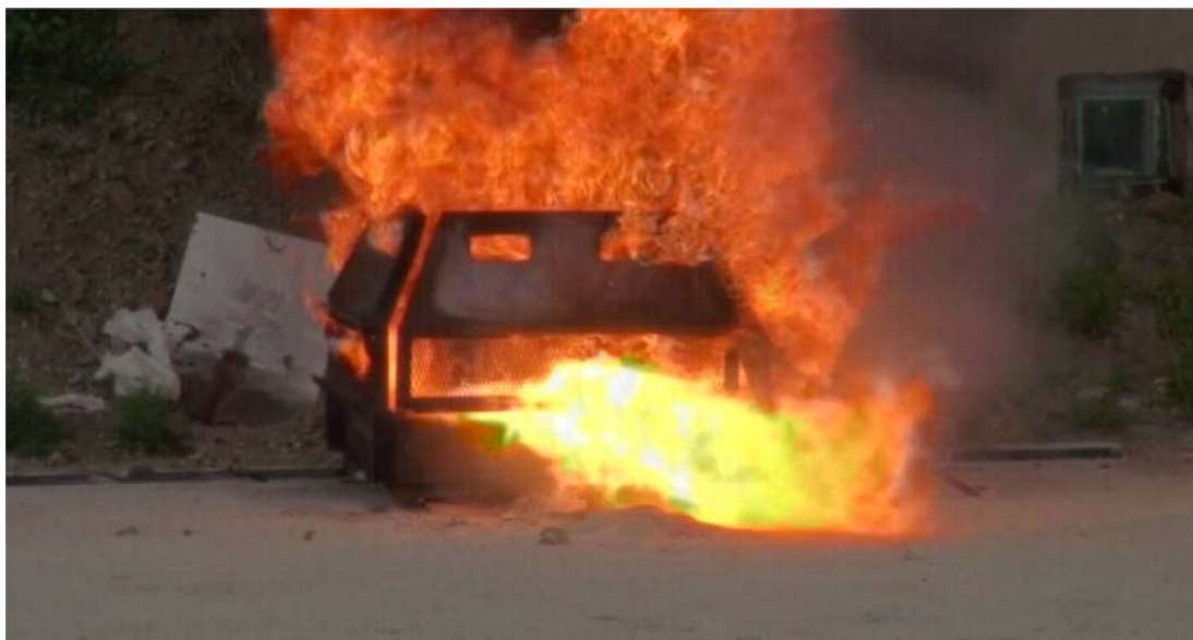
Figure 51. Deflagration of PBXN-109 Explosive, Test 7
