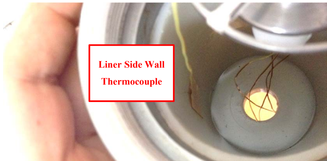
Figure 31. Surface Type Thermocouple That Is Located in the Middle of Test Item Sidewall
