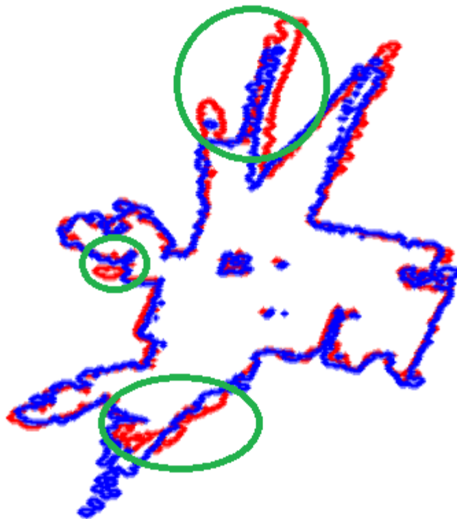
Figure 6-79 Achieved alignment between first height level (red), 53 cm, and second height level (blue), 66 cm, for Experiment-3
