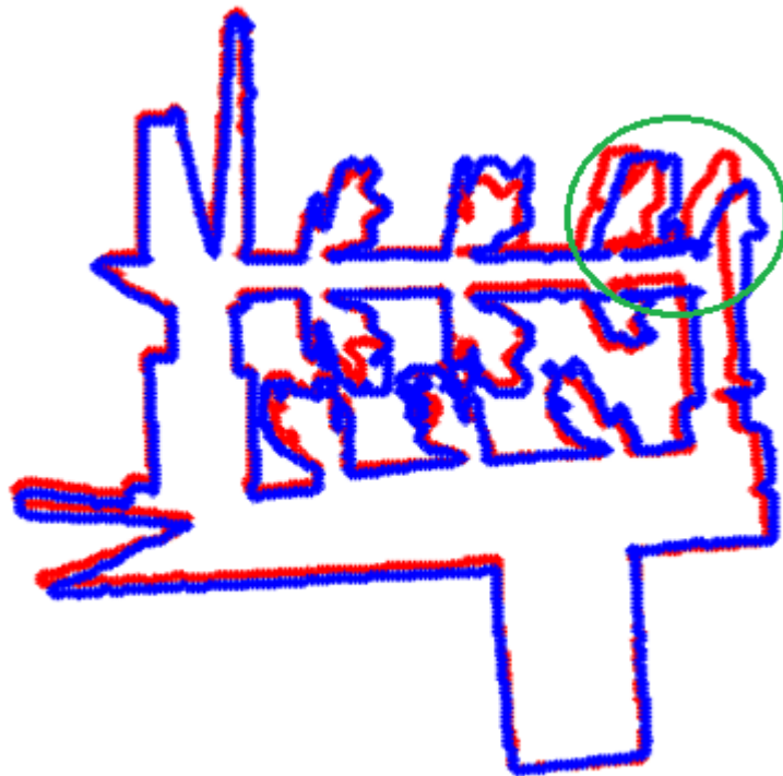
Figure 6-14 Achieved alignment between first height level (red), 81 cm, and second height level (blue), 86 cm, for Experiment-1
