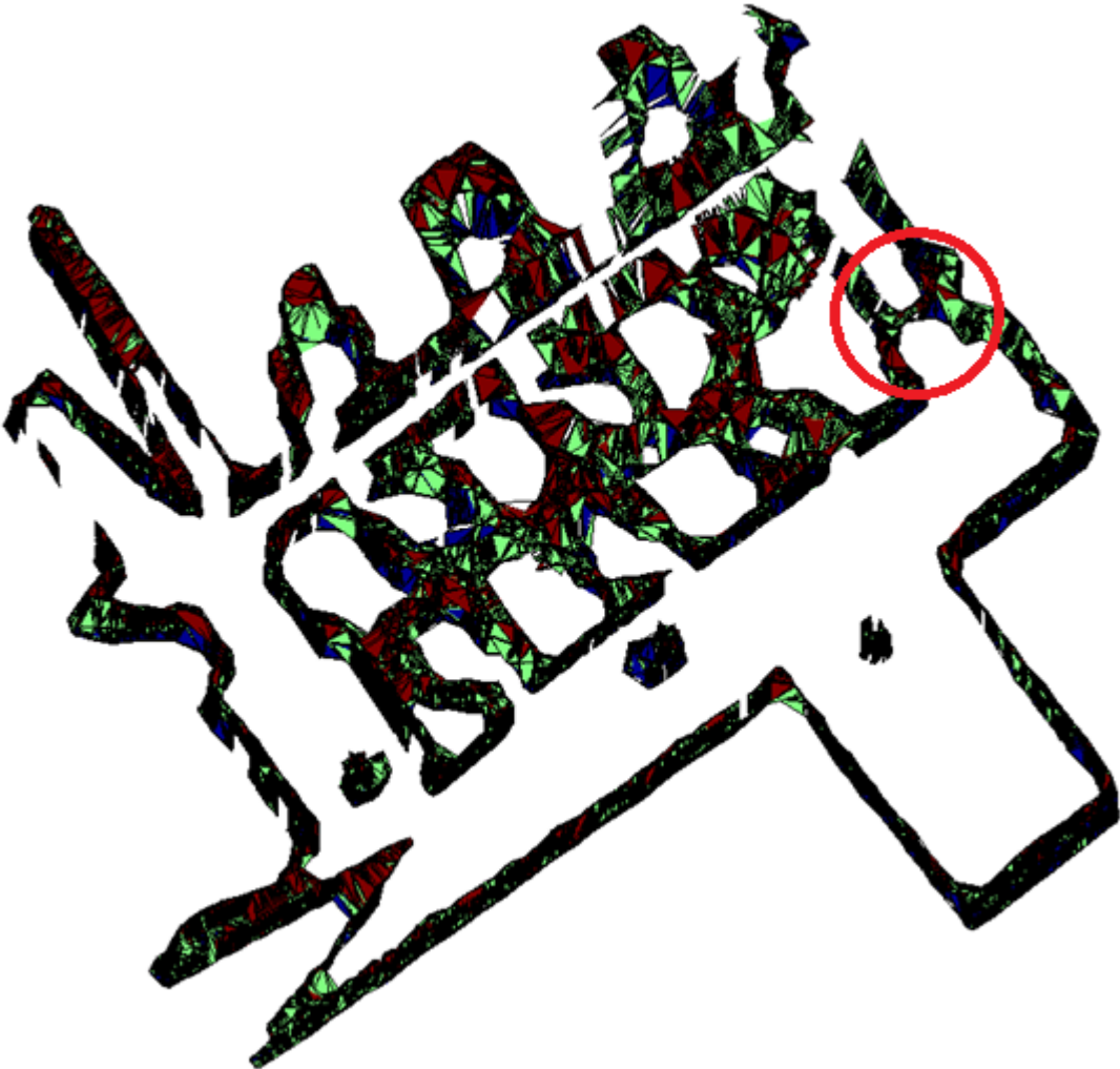
Figure 6-43 Tiling result for correspondence point sets of second height level, 86 cm, and third height level, 91 cm, added to the previous result for Experiment-1
