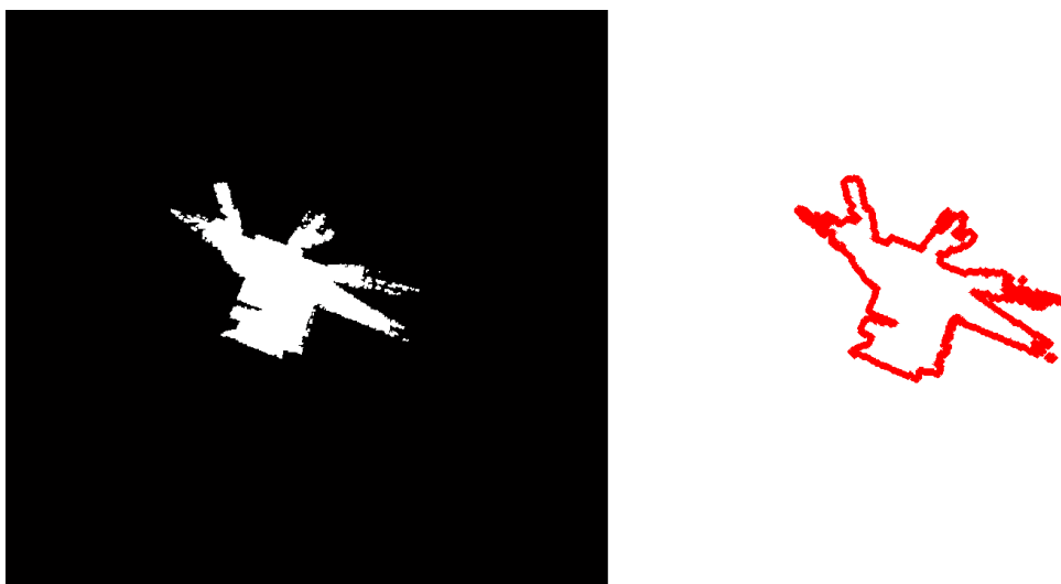
Figure 6-91 Similar regions of the third height level (left), 81 cm, and their generated correspondence point sets (right) for Experiment-3
