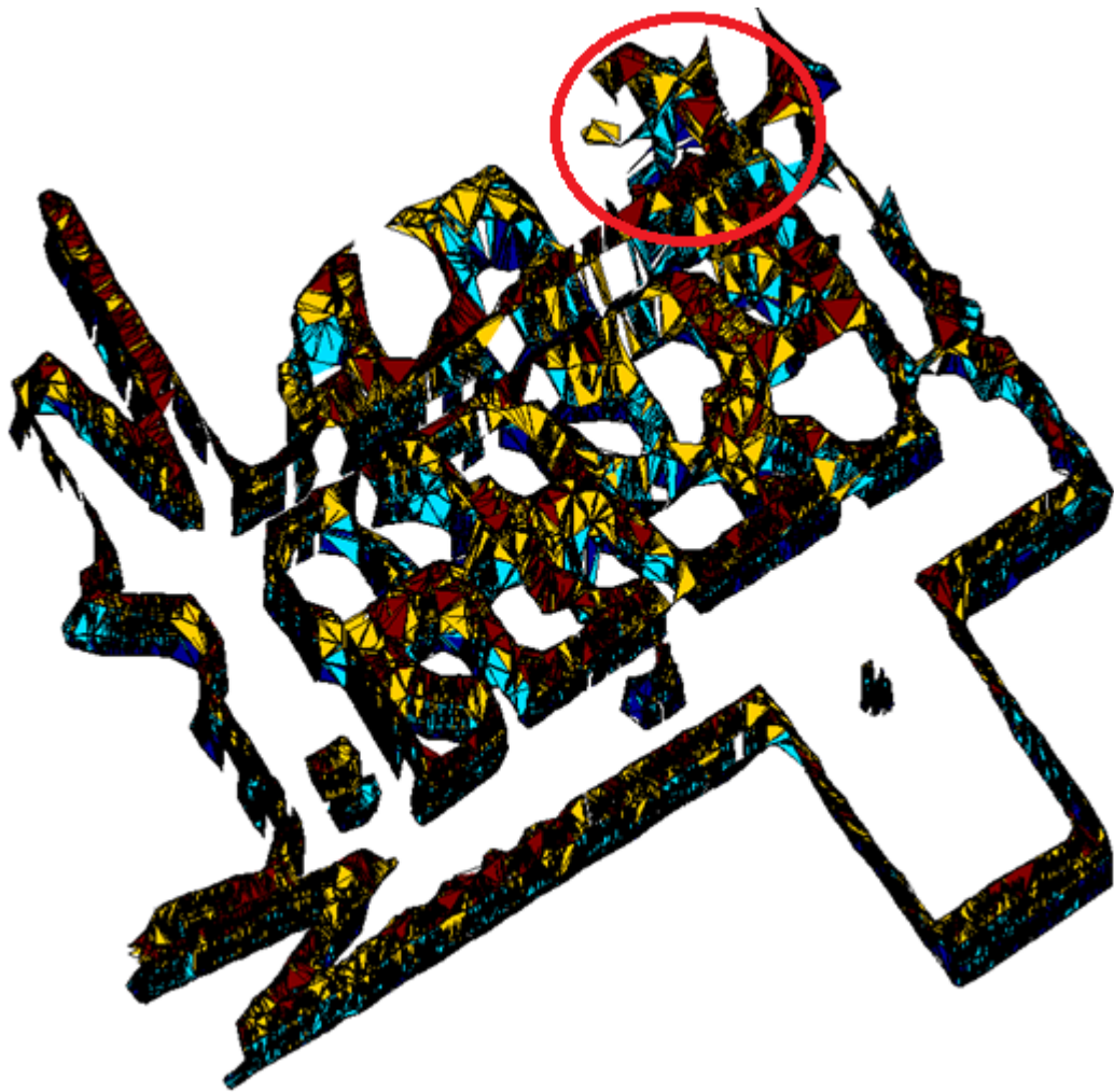
Figure 6-44 Tiling result for correspondence point sets of third height level, 91 cm, and fourth height level, 96 cm, added to the previous result for Experiment-1
