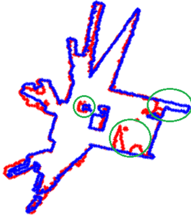
Figure 6-82 Achieved alignment between fourth height level (red), 86 cm, and fifth height level (blue), 91 cm, for Experiment-3
