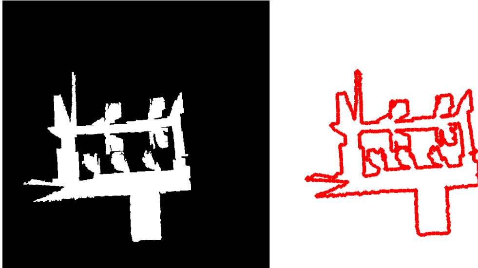
Figure 6-38 Similar regions of the fourth height level (left), 96 cm, and their generated correspondence point sets (right) for Experiment-1
