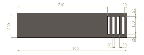
Figure 3.17 Grated bars only on the left part (All dimensions are in mm)
