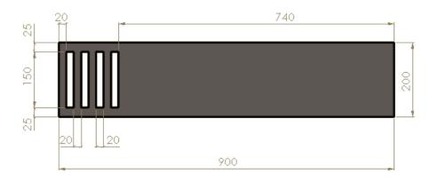
Figure 3.18 Grated bars only on the right part (All dimensions are in mm)
