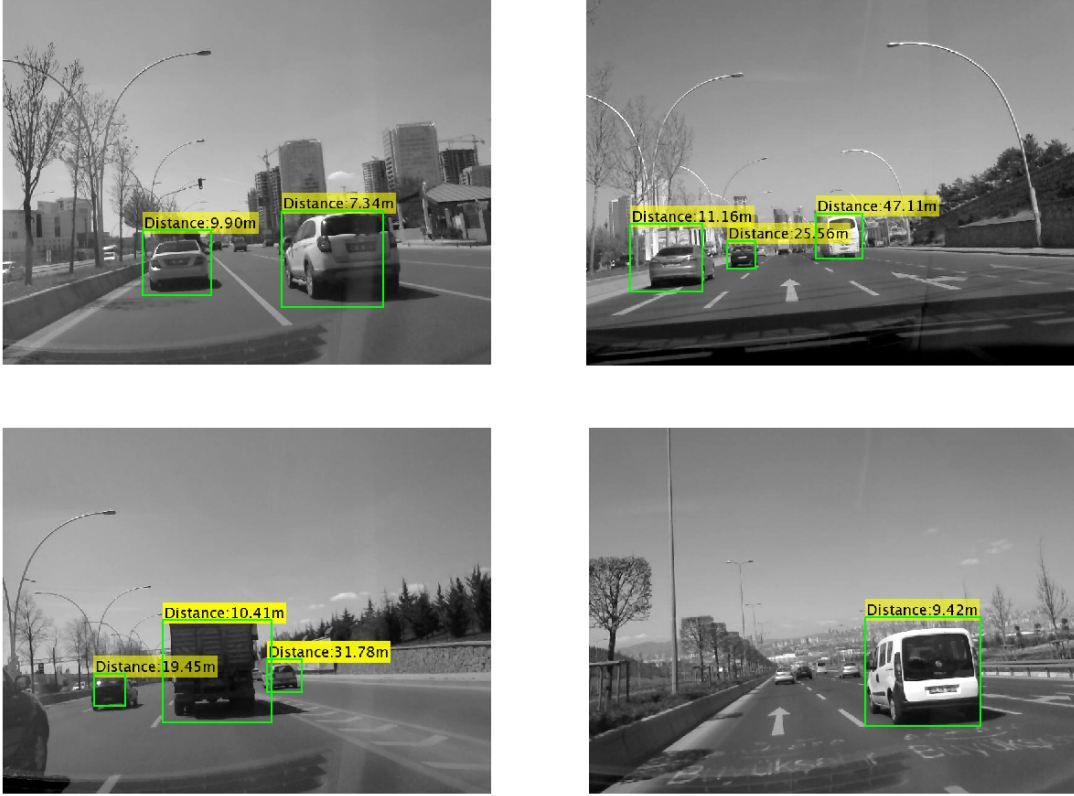
Figure 3.18: Correctly detected vehicles and their distances to the host vehicle in different frames
