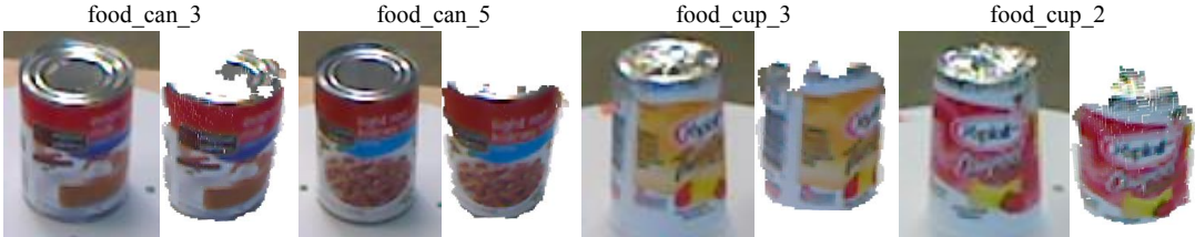
(a) Sensor fail to capture metallic surfaces.
