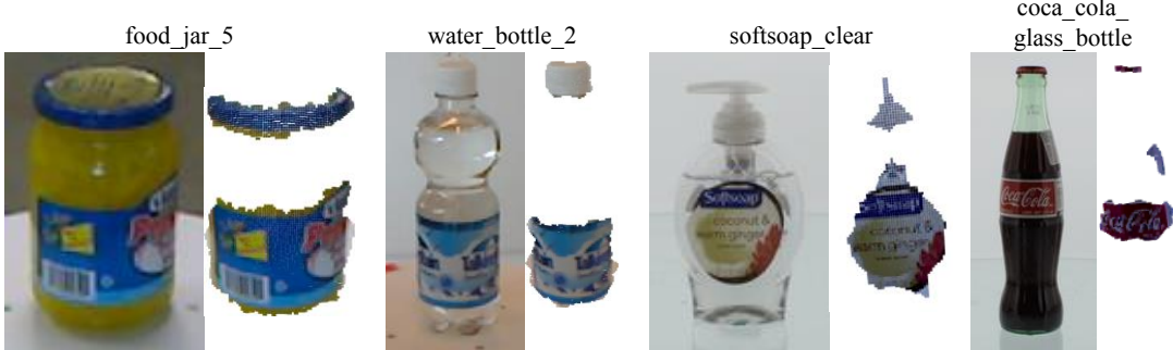
(b) Sensor fail to capture transparent surfaces.
