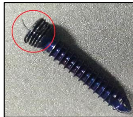
Figure 4.7 Failure of the threads of head in angled configuration.
