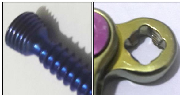
Figure 3.29 Close up views of the bone screw head and the connector. (Note the four-leaf clover shaped hole of connector)
