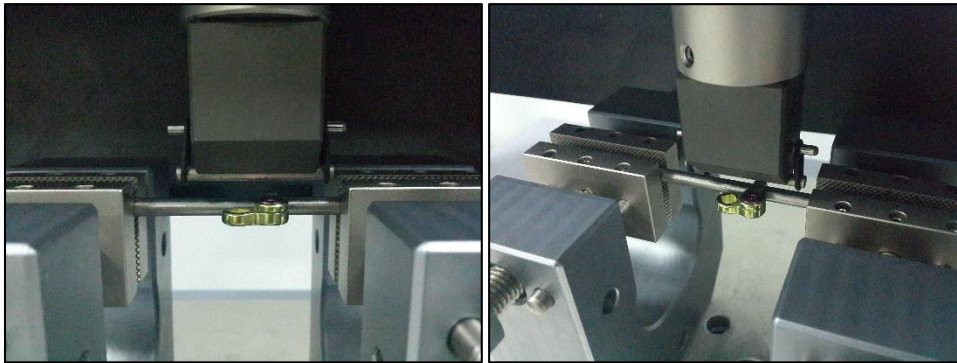
Figure 3.37 Placement of the rod and the connector during torsional gripping tests.
