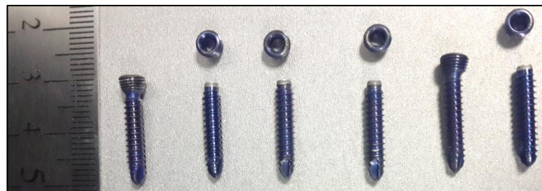
Figure 4.8 Failure modes of the bone screws after mechanical tests.
