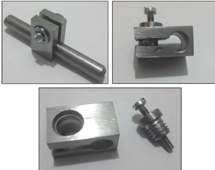
Figure 3.21 Pictures of the prototype of screw within screw concept.
