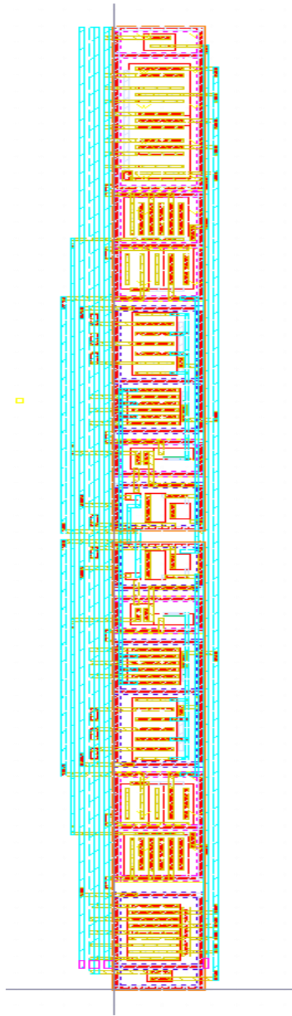
Figure 3-14: Layout of the single preamplifier. The height is 300 \mu\text{m} and the width is 35 \mu\text{m} .
