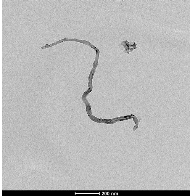
Figure C.2 TEM image of purified BNNT (P-BN-MO-2) synthesized using iron oxide at 1300°C
