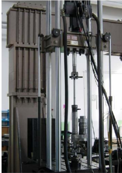
Figure 2.3: Test Rig for the Validation of the HP Suspension Model [3]
