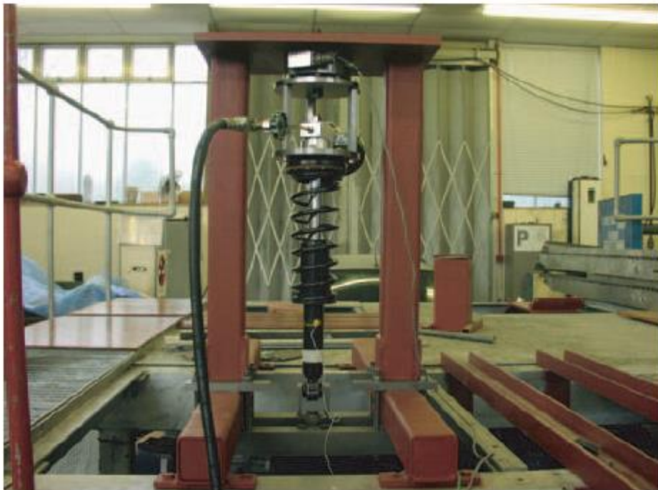
Figure 2.8: Test Rig for HP Suspension System [6]
