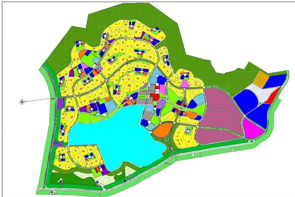
Figure 27: The discrete development plan of Urmia in Golman-Khane The yellow areas are representing the one or two story buildings, while violet areas are representing the housings with four stories Source: Consulting, Engineers of Arseh
