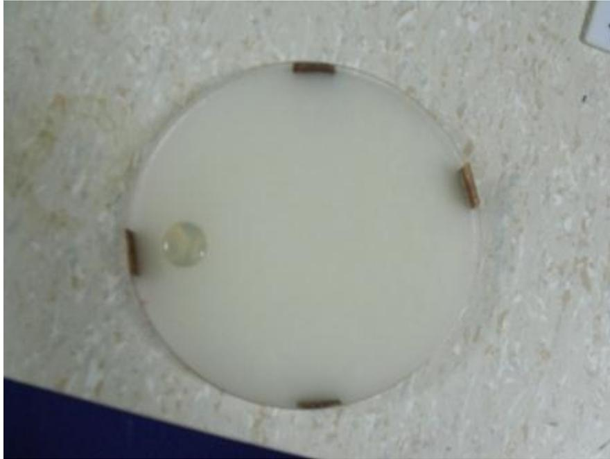
Fig. 4.7 Agar phantom sample picture. Copper electrodes are inserted to the boundary of the model and tumor tissue is located 1 cm away from the left side boundary.
