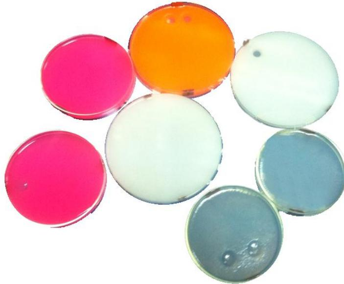
Fig. 4.8 Thermal-body phantoms used in experiments performed at Quantum Devices & Nanophotonics Research Lab. (Homogeneous and inhomogeneous phantoms including single or poly tumor tissues)
