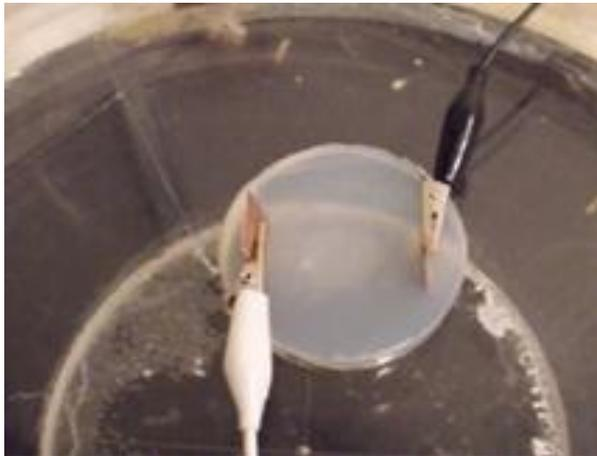
Fig. 4.9 Homogeneous agar phantom. Current is applied with copper electrodes located at right and left side of the phantom.
