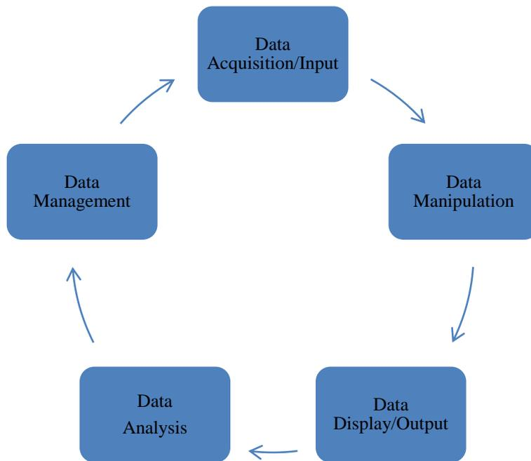
Figure 1. Components of GIS (adapted from Murray, 2009)
