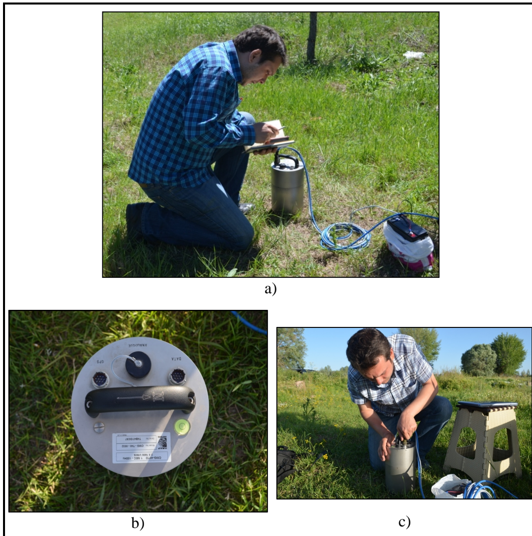
Figure 49. a) A view from the microtremor measurements at the Ort01 (2) site, b) a close-up view of the CMG-40TD velocimeter, c) A view from setting up the seismograph before the recording.
