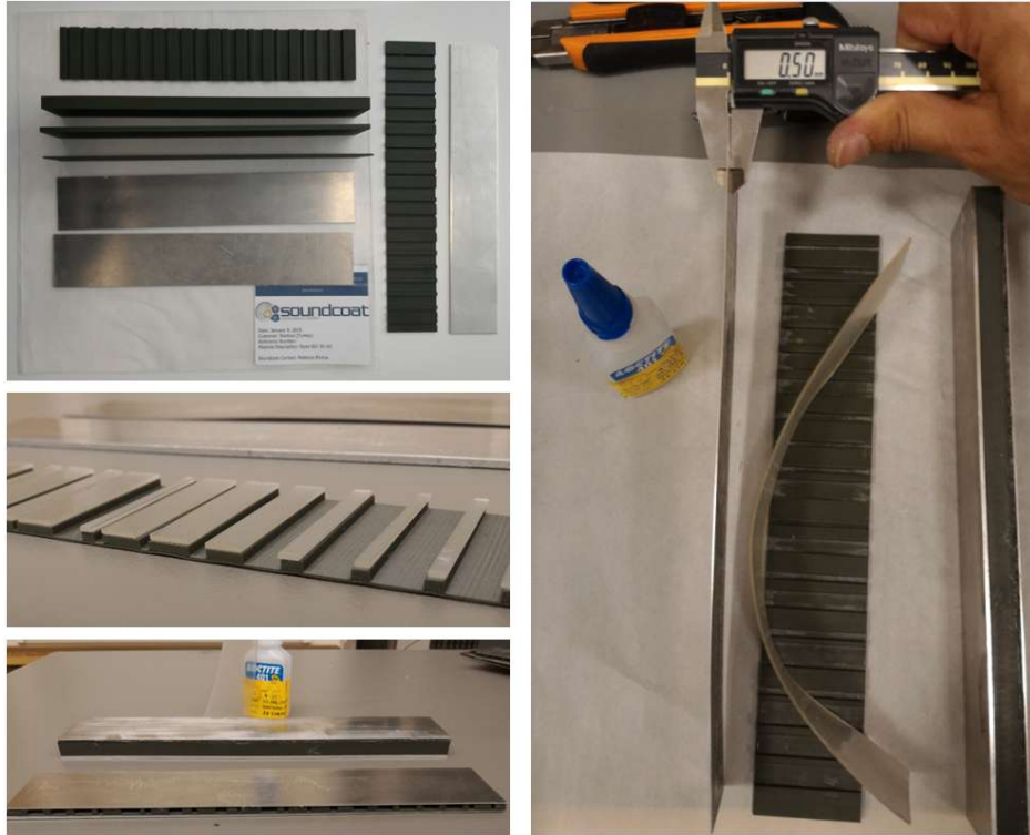
Figure 4-4 Assemblage of each individual layers to form treated beams
