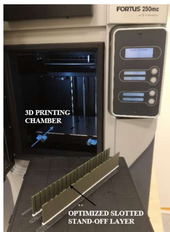
Figure 4-3 3D prototypes of optimized slotted stand-off layer
