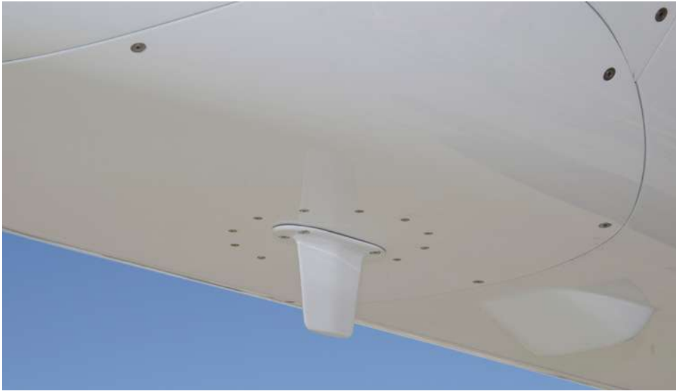
Figure 1-8 Blade antenna attached to the skin of an aircraft [11]
