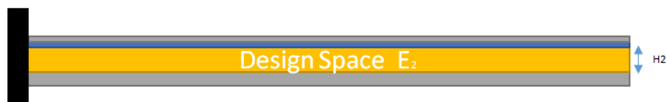
Figure 3-84 Cantilever sandwich beam model and its design variables ( E_2 & H_2 )
